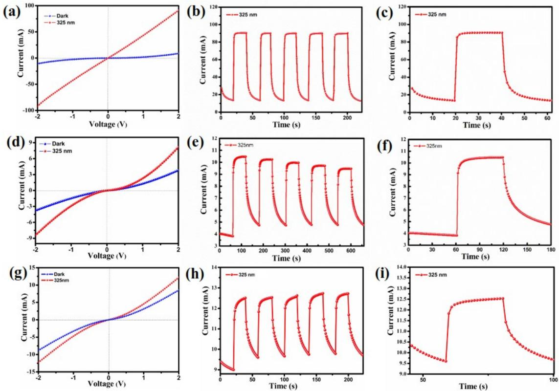
Figure S3. The I-V curves of photodetectors based on porous GaN annealed at (a) 900°C, (d) 1100°C, and (g) 1200°C, respectively. Time responses of the photodetectors based on porous GaN annealing at (b) 900°C, (e) 1100°C, and (h) 1200°C, respectively. Enlarge view of the current rise and decay processes of the photodetectors based on porous GaN annealed at (c) 900°C, (f) 1100°C, and (i) 1200°C, respectively.
