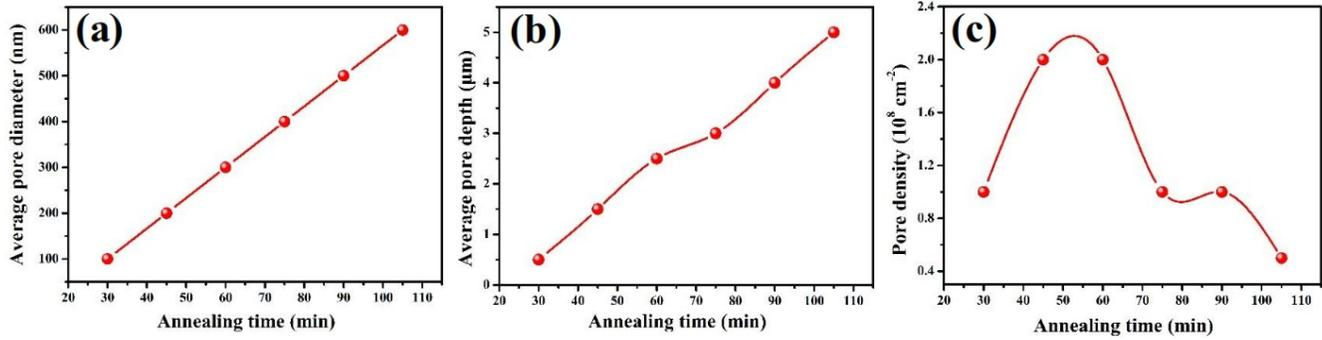
Figure S2. Average pore diameter (a), average pore depth (b), and pore density (c) of porous GaN plotted as a function of annealing time at 1150°C.
