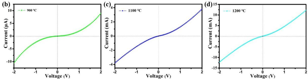
Figure S5 Enlarged view of the dark current of the UV photodetectors based on porous GaN annealing at (b) 900 °C, (c) 1100 °C, and (d) 1200 °C, respectively.
