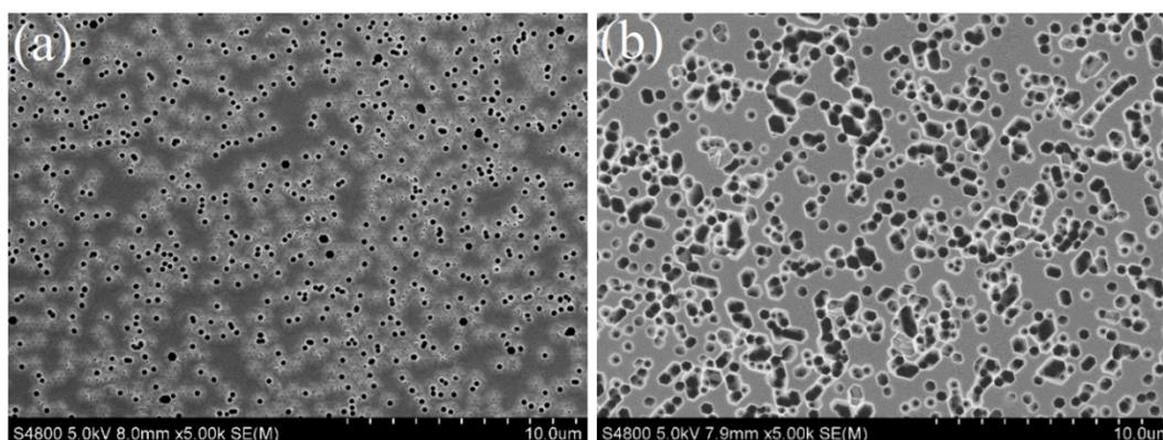
Figure S1. SEM images of GaN samples annealed at (a) 1050°C, (b) 1150°C for 60 min.
