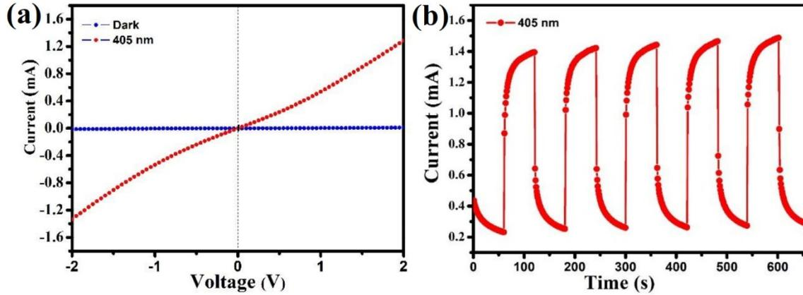
Figure S4. (a) The  $I$ - $V$  curves of porous GaN (annealing at 1000°C) device under dark and UV-light illumination with 405 nm laser. (c) Time response ( $I$ - $t$  curve) of the porous GaN (annealing at 1000°C) photodetector with 405nm laser.
