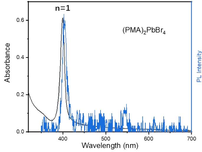
**Figure S2.** UV-vis absorption and PL spectra of  $(\text{PMA})_2\text{PbBr}_4$  film.
