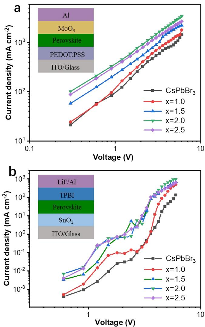
**Figure S1.** Current density–voltage curves for (a) hole-only and (b) electron-only devices. Inset: device configurations of the hole-only and electron-only devices.
