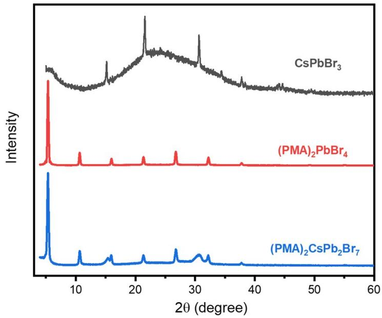
**Figure S3.** XRD profiles of  $\text{CsPbBr}_3$ ,  $(\text{PMA})_2\text{PbBr}_4$  and  $(\text{PMA})_2\text{CsPb}_2\text{Br}_7$  perovskites.
