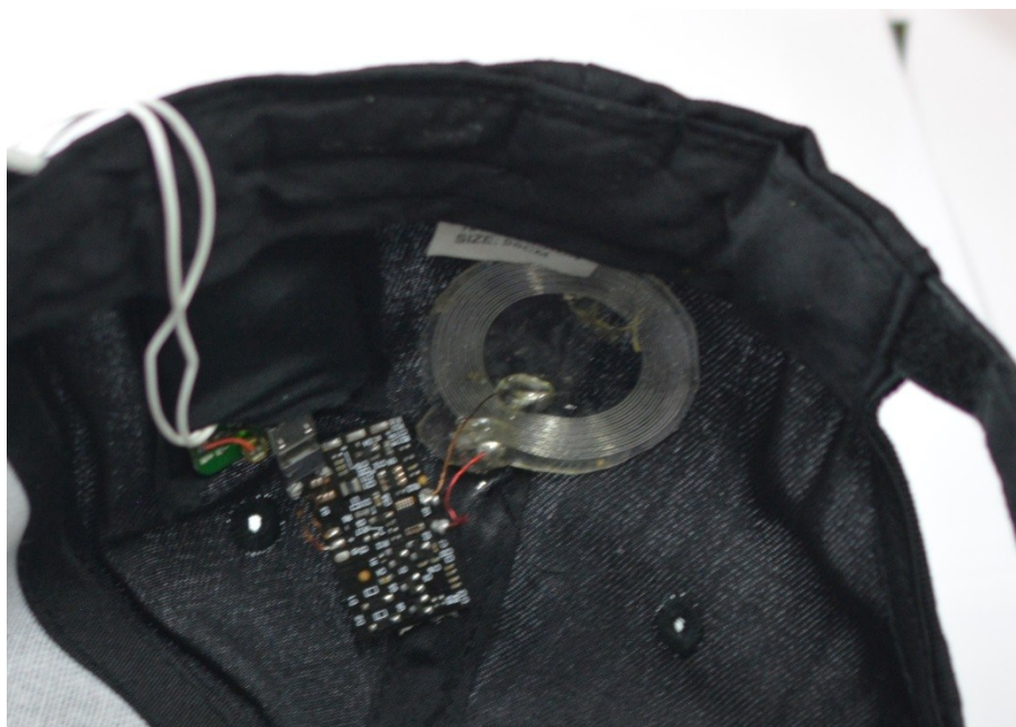
Figure S11. Digital image of a bluetooth hat equipped with a wireless receiver.
