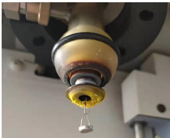
**Fig. S3** Picture of TGA crucible after the heating and cooling process of TCNQ.
