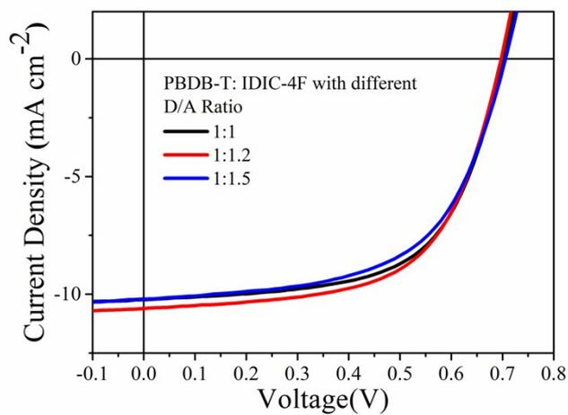
**Table S4.** Photovoltaic properties of the PSCs based on PBDB-T: IDIC-4F with different D/A Ratio.
