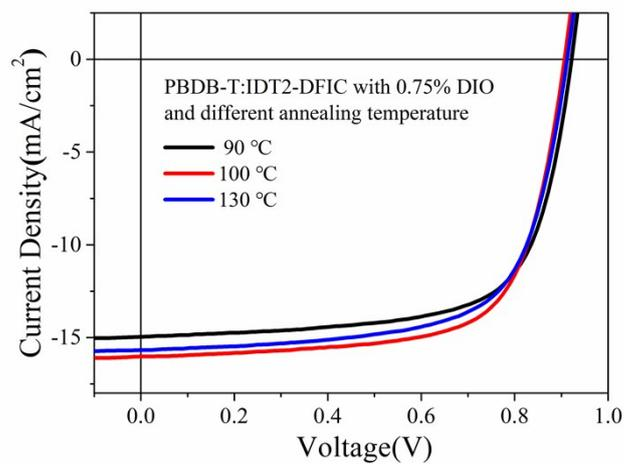
**Table S3.** Photovoltaic properties of the PSCs based on PBDB-T: IDT2-DFIC with different annealing temperature.
