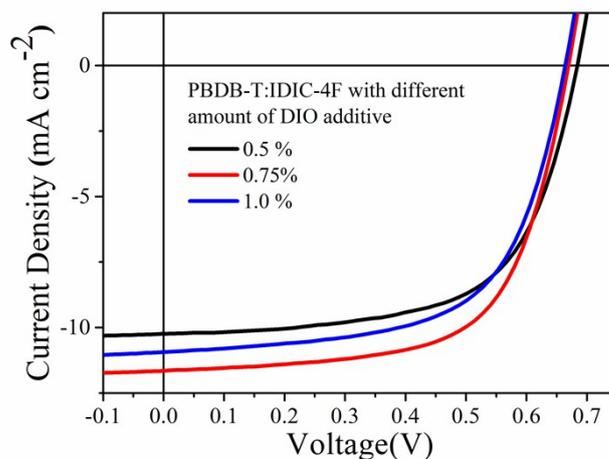
**Table S6.** Photovoltaic properties of the PSCs based on PBDB-T: IDIC-4F with different amount of DIO additive.
