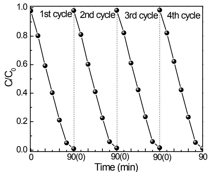
Figure S8. The cyclic photocatalytic phenol degradation test of  $\text{ZnO}/\text{Ag}/\text{Ag}_2\text{O}$  under white light irradiation.
