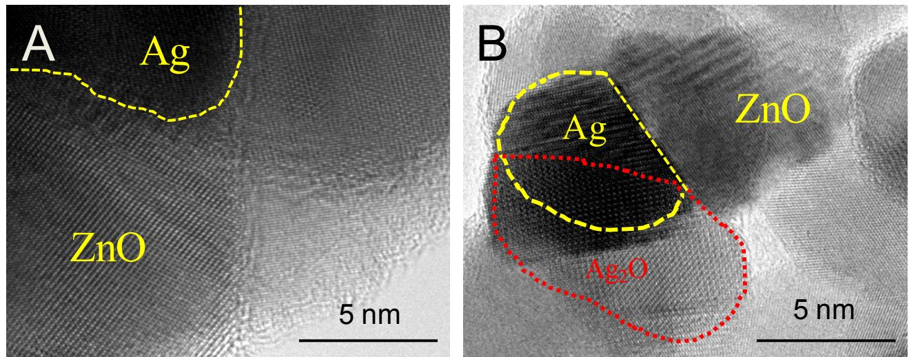
Figure S4. HRTEM images of  $\text{ZnO}/\text{Ag}$  (A) and  $\text{ZnO}/\text{Ag}/\text{Ag}_2\text{O}$  (B).
