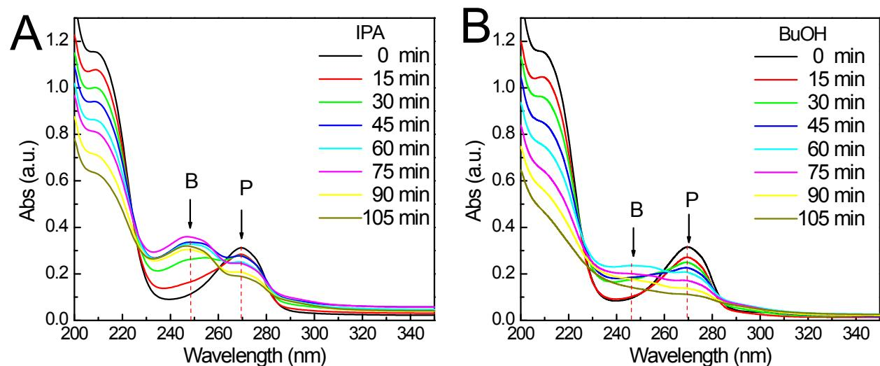
Figure S9. UV absorption spectra of phenol illuminated by white light for various durations in the presence of ZnO/Ag/Ag<sub>2</sub>O containing with IPA (A) or BuOH (B).
