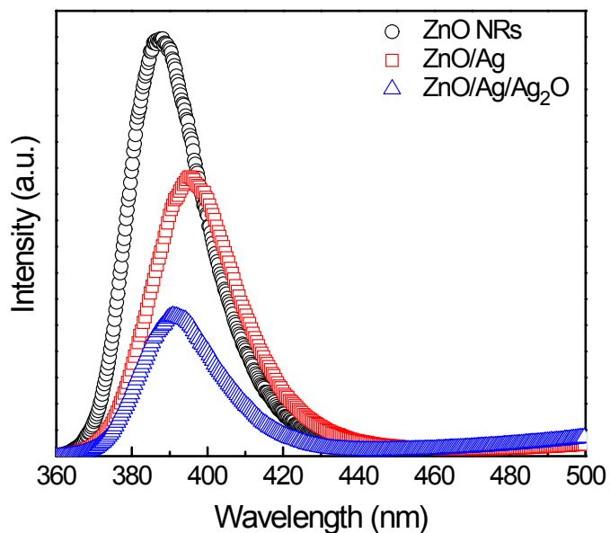
Figure S6. Micro-photoluminescence spectra of ZnO NRs, ZnO/Ag and ZnO/Ag/Ag<sub>2</sub>O.
