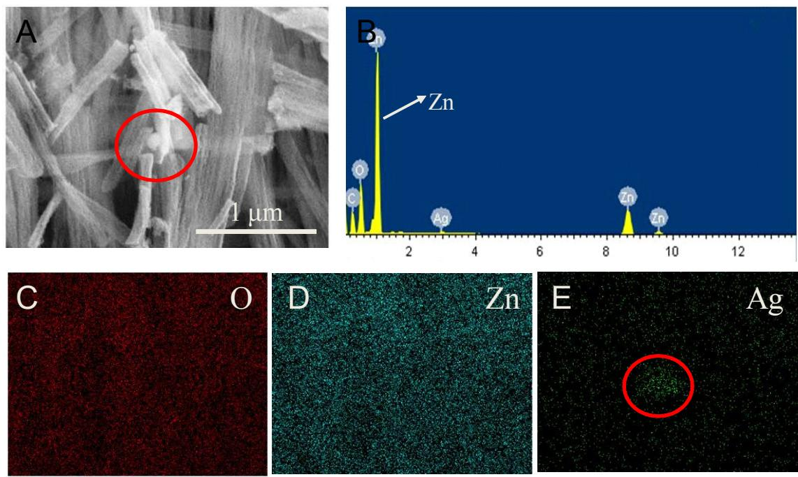
Figure S3. The SEM image (A), EDS spectrum (B) and EDS elemental mapping (C: Oxygen, D: Zinc, E: Silver) of  $\text{ZnO}/\text{Ag}/\text{Ag}_2\text{O}$ .
