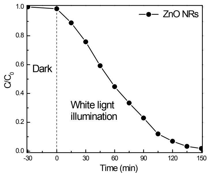
Figure S5. Effect of ZnO NRs photocatalyst on phenol degradation under white light illumination.
