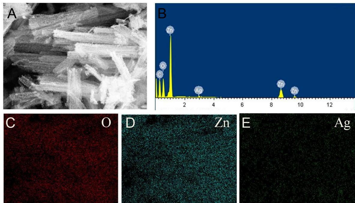
Figure S2. The SEM image (A), EDS spectrum (B) and EDS elemental mapping (C: Oxygen, D: Zinc, E: Silver) of ZnO/Ag.
