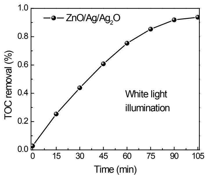
Figure S7. TOC removal efficiency in the presence of  $\text{ZnO}/\text{Ag}/\text{Ag}_2\text{O}$  under white light irradiation.
