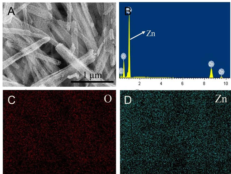
Figure S1. The SEM image (A), EDS spectrum (B) and EDS elemental mapping (C: Oxygen, D: Zinc) of ZnO NRs.
