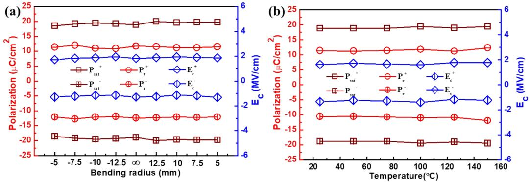
Figure S5. (a) Variations of  $P_{sat}$ ,  $P_r$ , and  $E_c$  of flexible HZO films under stress and electric field conditions and (b) under temperature and electric field conditions.
