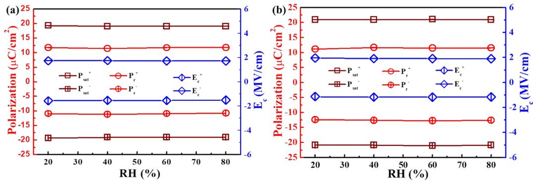
Figure S8. variations of  $P_{sat}$ ,  $P_r$ , and  $E_c$  of the P-E hysteresis loops of the flexible HZO films (a) under humidity and electric field conditions, (d) under humidity, high temperature and electric field conditions.
