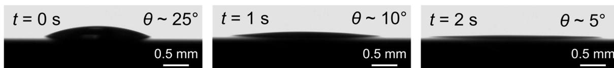
**Fig. S1** – Wetting of PZT ink on platinized silicon. A  $\sim 1 \mu\text{L}$  droplet was deposited on a platinized silicon substrate degassed at  $350 \text{ }^\circ\text{C}$  for 5 min. Complete wetting occurs within seconds.
