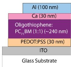
**Figure S9.1:** Schematic of OPV device architecture
