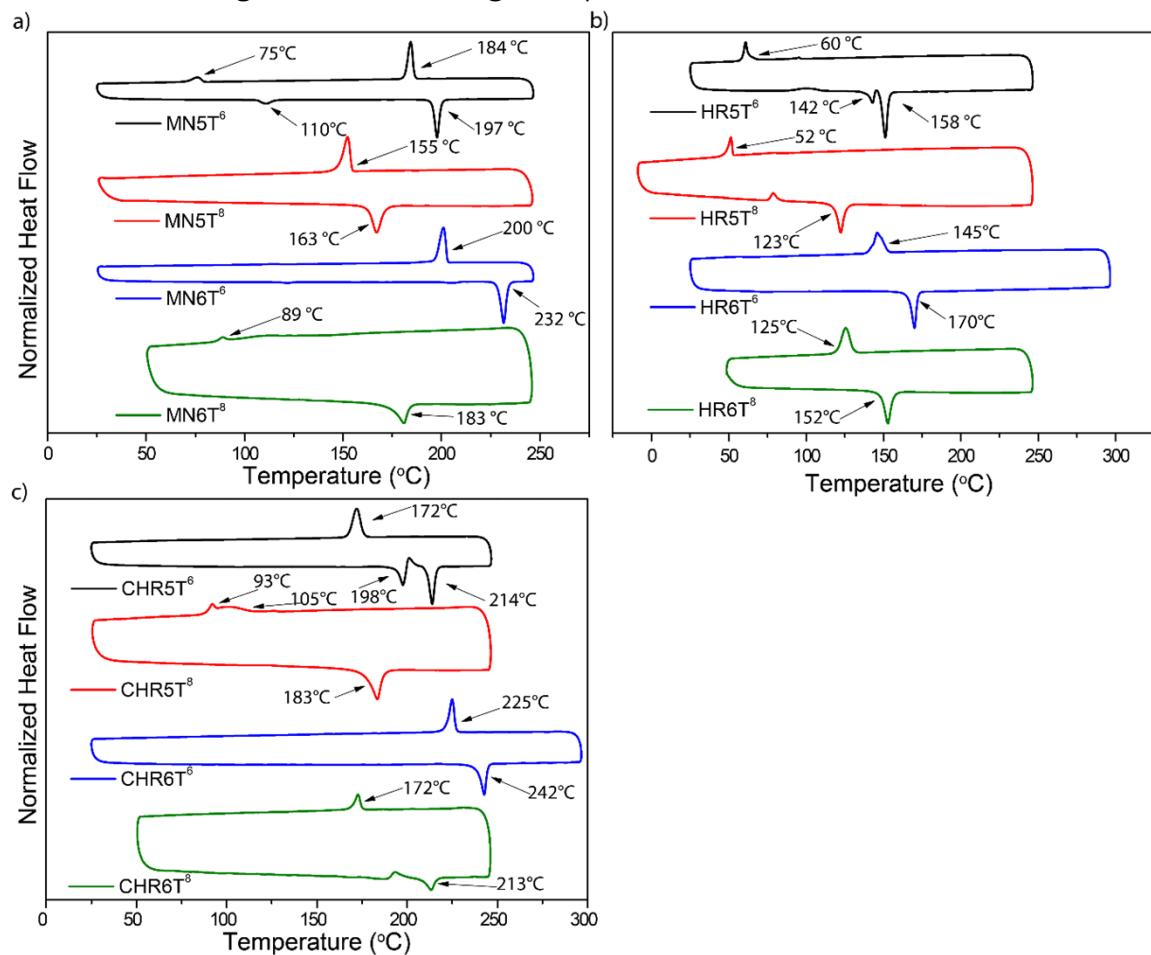
**Figure S6.1.** Normalized DSC thermograms for our oligothiophene materials with a) **MN-**, b) **HR-** and c) **CHR-** end-group acceptors with labelled phase transition temperatures
