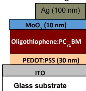
**Figure S10.1:** Schematic of OPV device architecture
