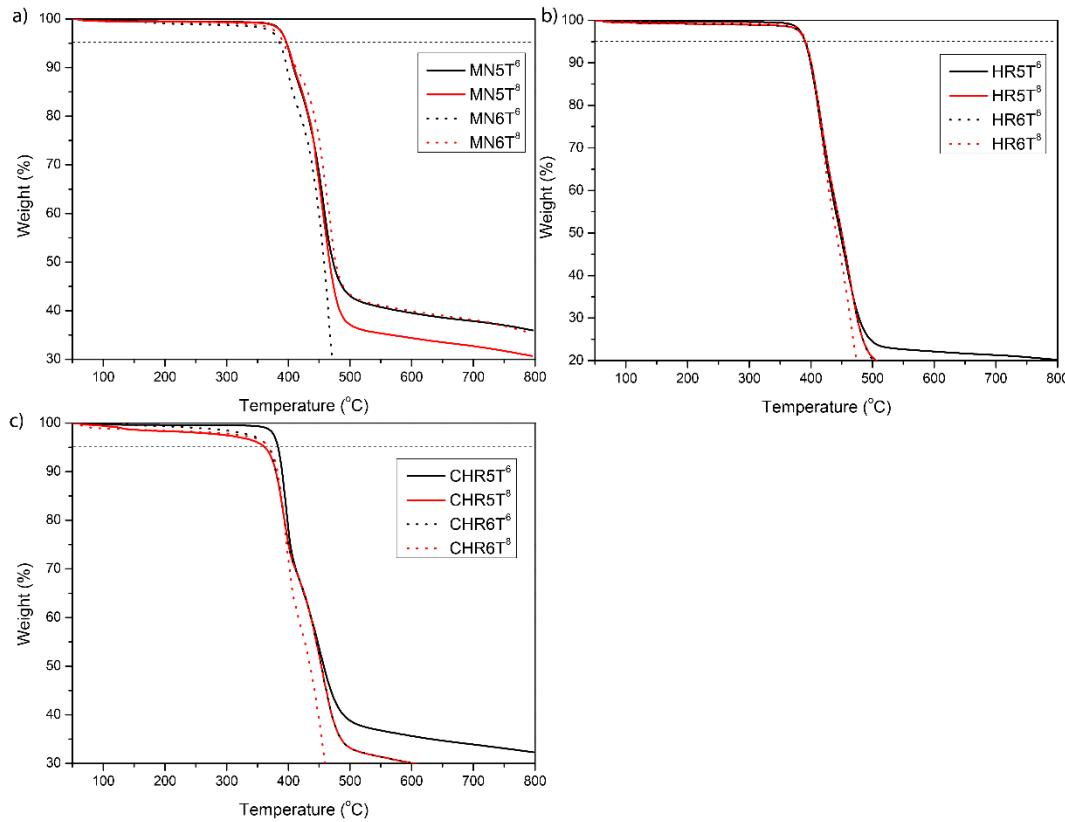
**Figure S5.1.** TGA thermograms of our oligothiophene materials with a) **MN-**, b) **HR-** and c) **CHR-** end-group acceptors.
