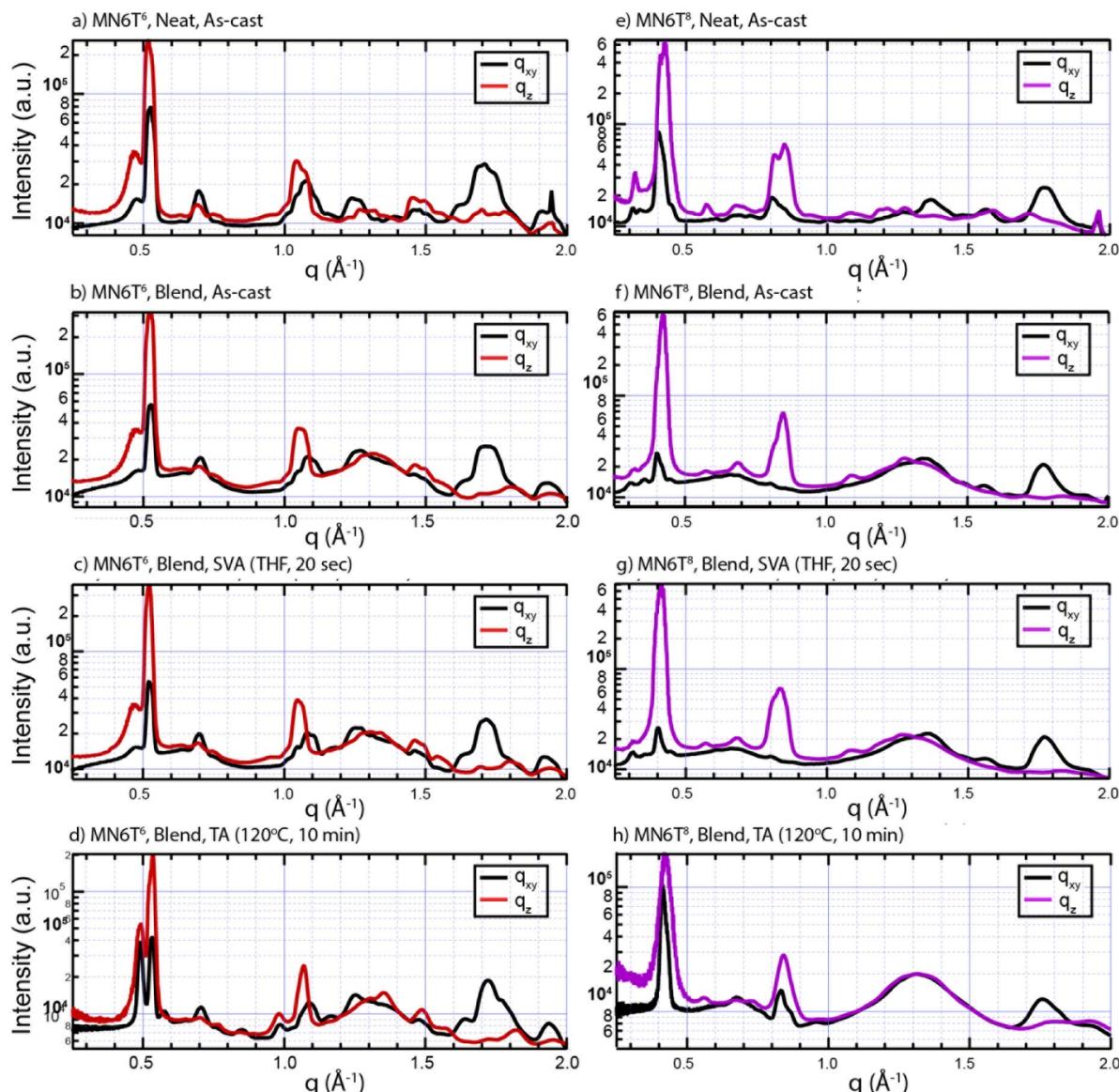
**Figure S11.2** Linecuts of the GIWAXS scattering patterns for the **MN6T<sup>6</sup>** (a-d) and **MN6T<sup>8</sup>** (e-h) materials of peak intensity along the horizontal ( $q_{xy}$ ) and vertical ( $q_z$ ) axes.
