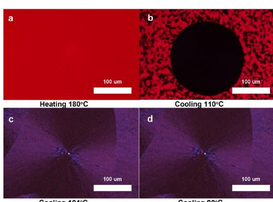
**Figure S6.5.** Selected POM images for **CHR5T<sup>8</sup>**, heating and cooling cycle
