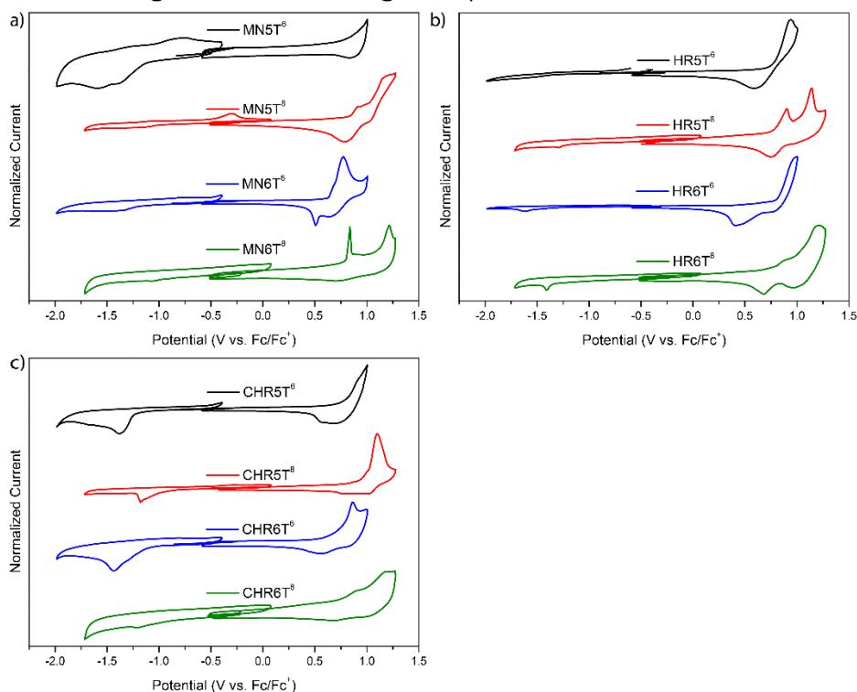
**Figure S8.1:** Normalized thin film cyclic voltammograms of our oligothiophene materials with a) **MN-**, b) **HR-** and c) **CHR-** end-group acceptors.
