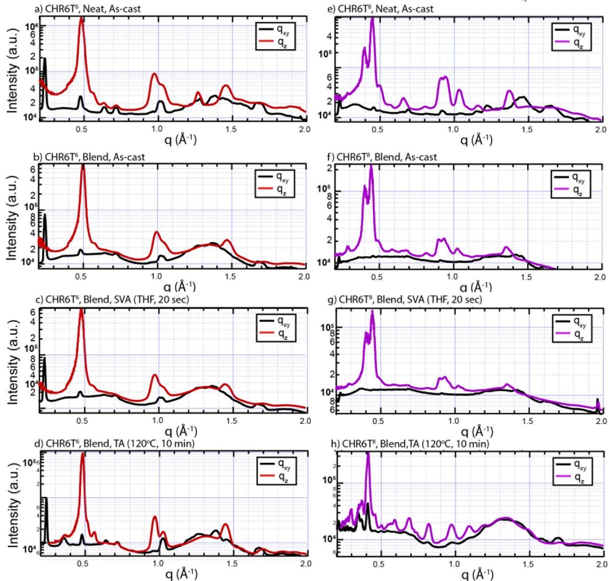
**Figure S11.6** Linecuts of the GIWAXS scattering patterns for the **CHR6T<sup>6</sup>** (a-d) and **CHR6T<sup>8</sup>** (e-h) materials of peak intensity along the horizontal ( $q_{xy}$ ) and vertical ( $q_z$ ) axes.
