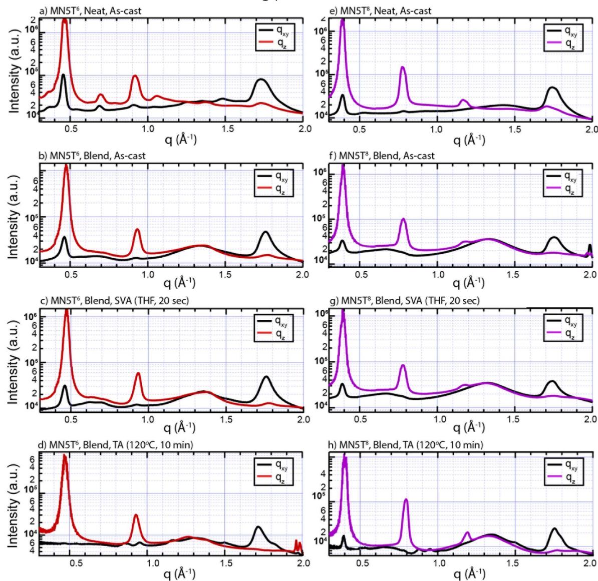
**Figure S11.1** Linecuts of the GIWAXS scattering patterns for the **MN5T<sup>6</sup>** (a-d) and **MN5T<sup>8</sup>** (e-h) materials of peak intensity along the horizontal ( $q_{xy}$ ) and vertical ( $q_z$ ) axes.
