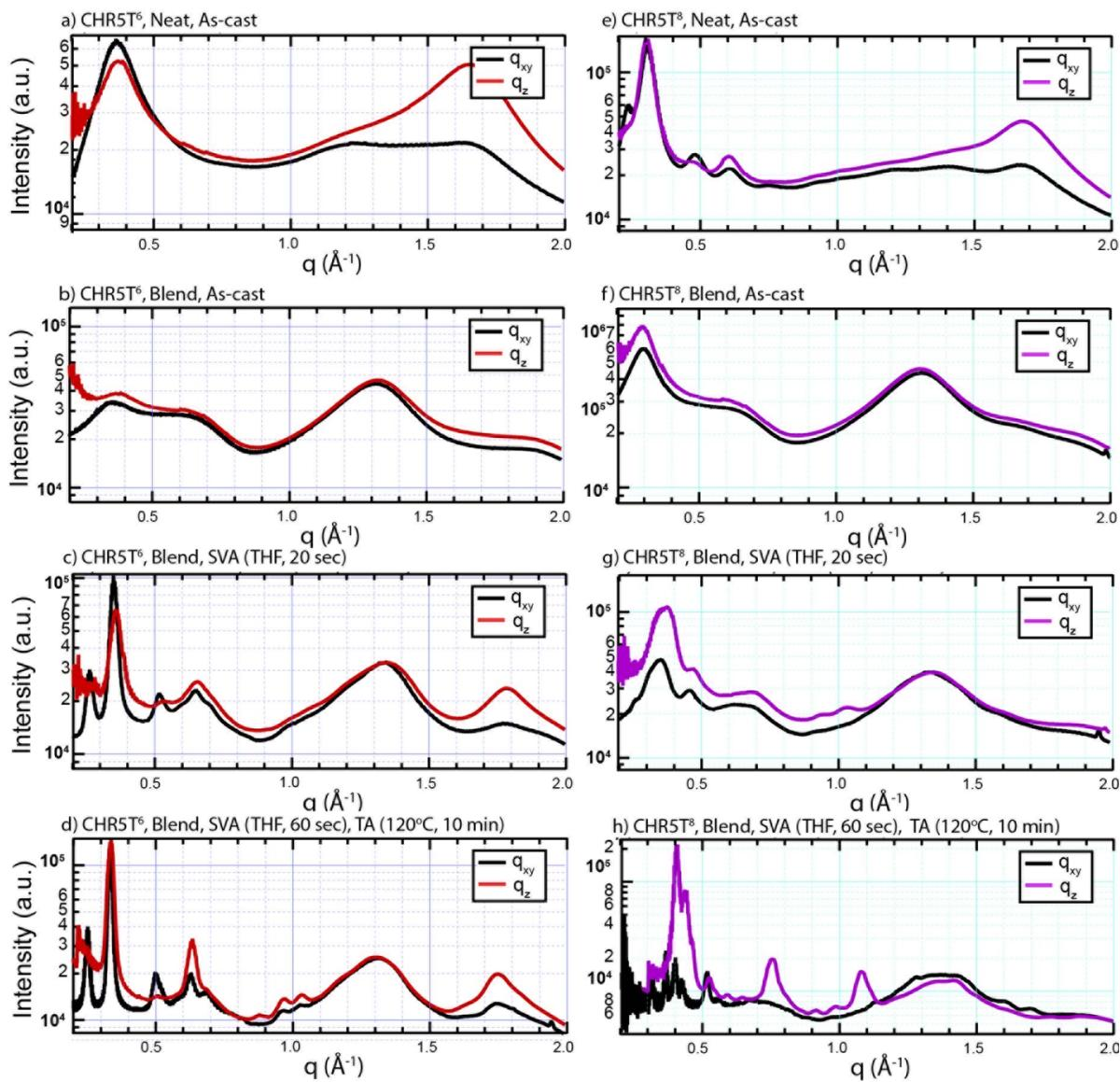
**Figure S11.5** Linecuts of the GIWAXS scattering patterns for the **CHR5T<sup>6</sup>** (a-d) and **CHR5T<sup>8</sup>** (e-h) materials of peak intensity along the horizontal ( $q_{xy}$ ) and vertical ( $q_z$ ) axes.
