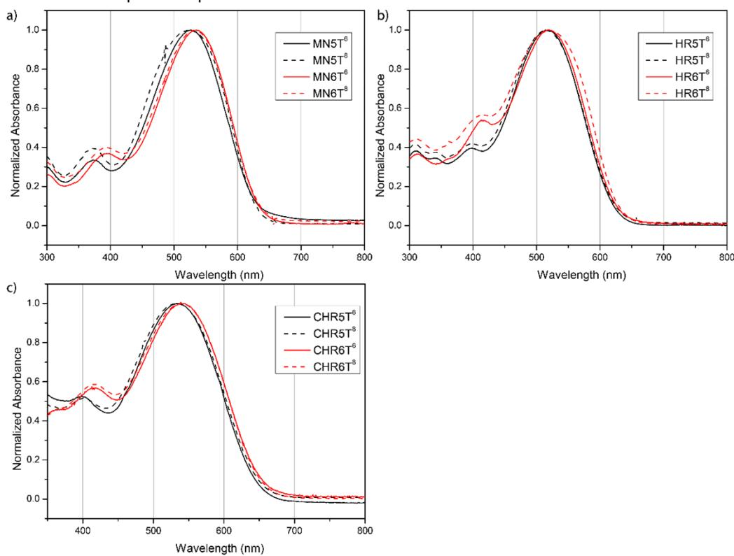
**Figure S7.1:** Normalized UV-vis absorption spectra of our oligothiophene materials with a) **MN-**, b) **HR-** and c) **CHR-** end-group acceptors, in chloroform solutions.
