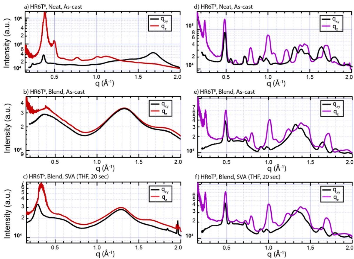
**Figure S11.4** Linecuts of the GIWAXS scattering patterns for the **HR6T<sup>6</sup>** (a-c) and **HR6T<sup>8</sup>** (d-f) materials of peak intensity along the horizontal ( $q_{xy}$ ) and vertical ( $q_z$ ) axes.
