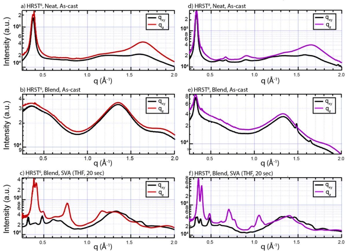
**Figure S11.3** Linecuts of the GIWAXS scattering patterns for the **HR5T<sup>6</sup>** (a-c) and **HR5T<sup>8</sup>** (d-f) materials of peak intensity along the horizontal ( $q_{xy}$ ) and vertical ( $q_z$ ) axes.
