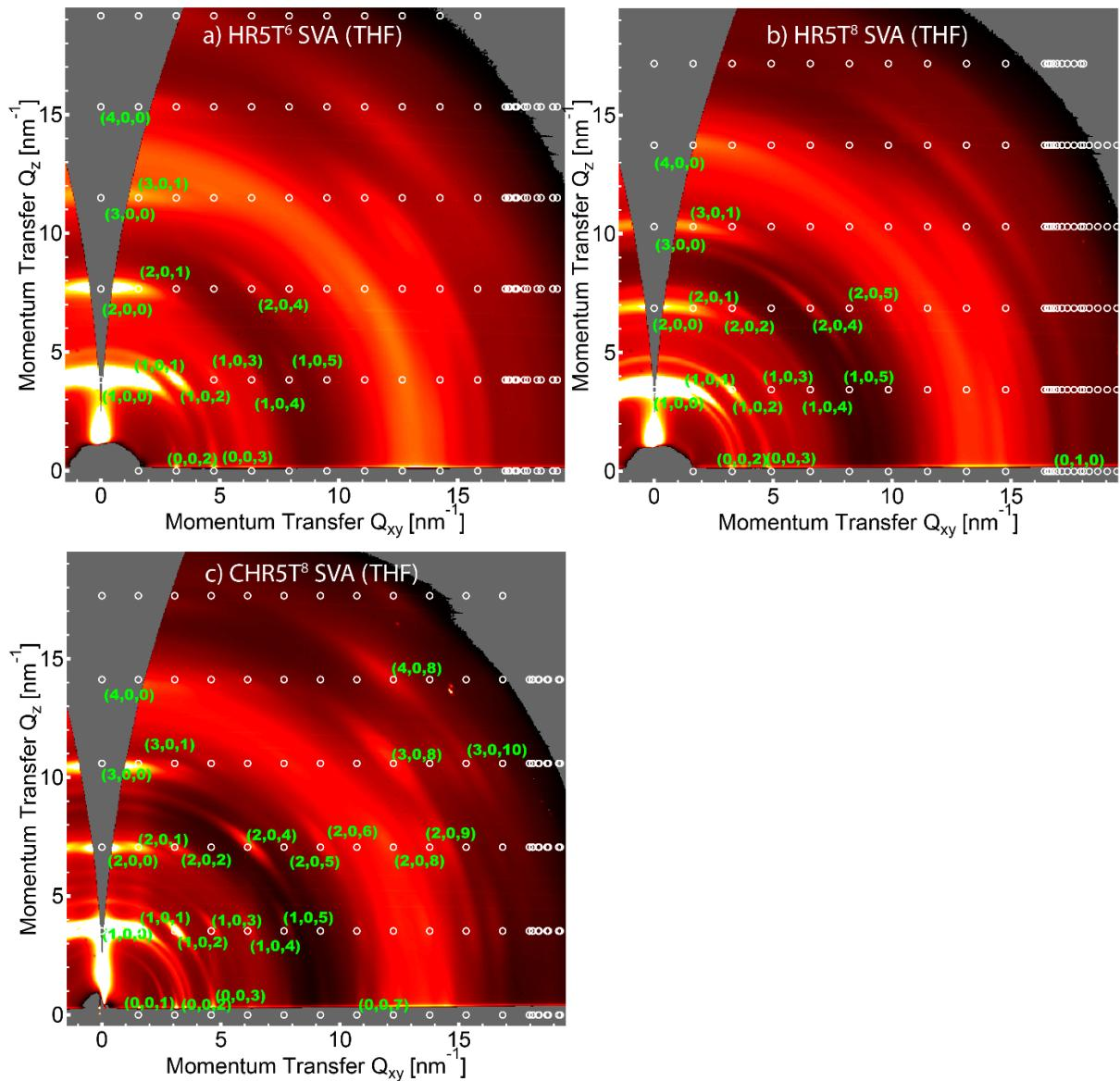
**Figure S11.7** Overlay of calculated lattices points (white circles) onto experimental GIWAXS patterns of a) HR5T<sup>6</sup>, b) HR5T<sup>8</sup> and c) CHR5T<sup>8</sup>. Unit cell parameters are given earlier.
