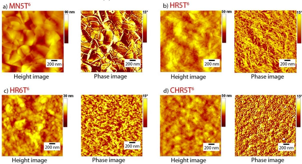
**Figure S12.1** AFM images showing the surface topography of the annealed blend films of a) **MN5T<sup>6</sup>**, b) **HR5T<sup>6</sup>**, c) **HR6T<sup>6</sup>** and d) **CHR5T<sup>6</sup>**. Annealing conditions and film blend composition are identical to those that give the best OPV device performance.
