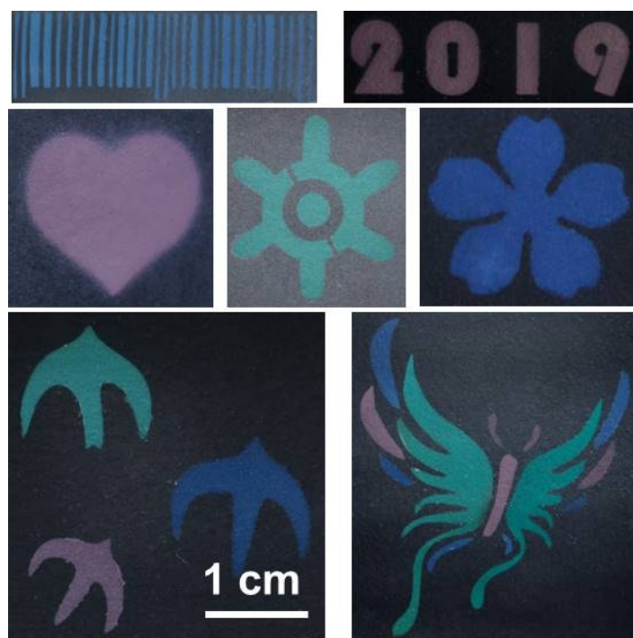
Figure S6. Diverse pattern design of the structural color anti-counterfeiting label by the facile spray-coating method.
