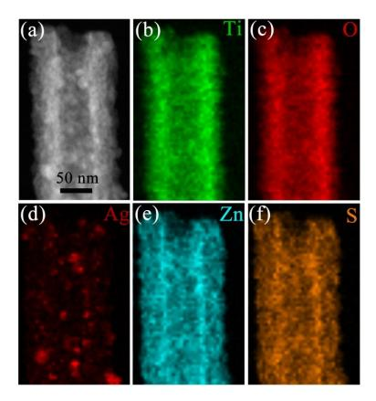
Fig. S1 (a) HAADF-STEM image of a  $TiO_2/Ag/ZnS$  nanotube and corresponding EDS mapping images for Ti (b), O (c), Ag (d), Zn (e) and S (f) of the same nanotube, respectively.
