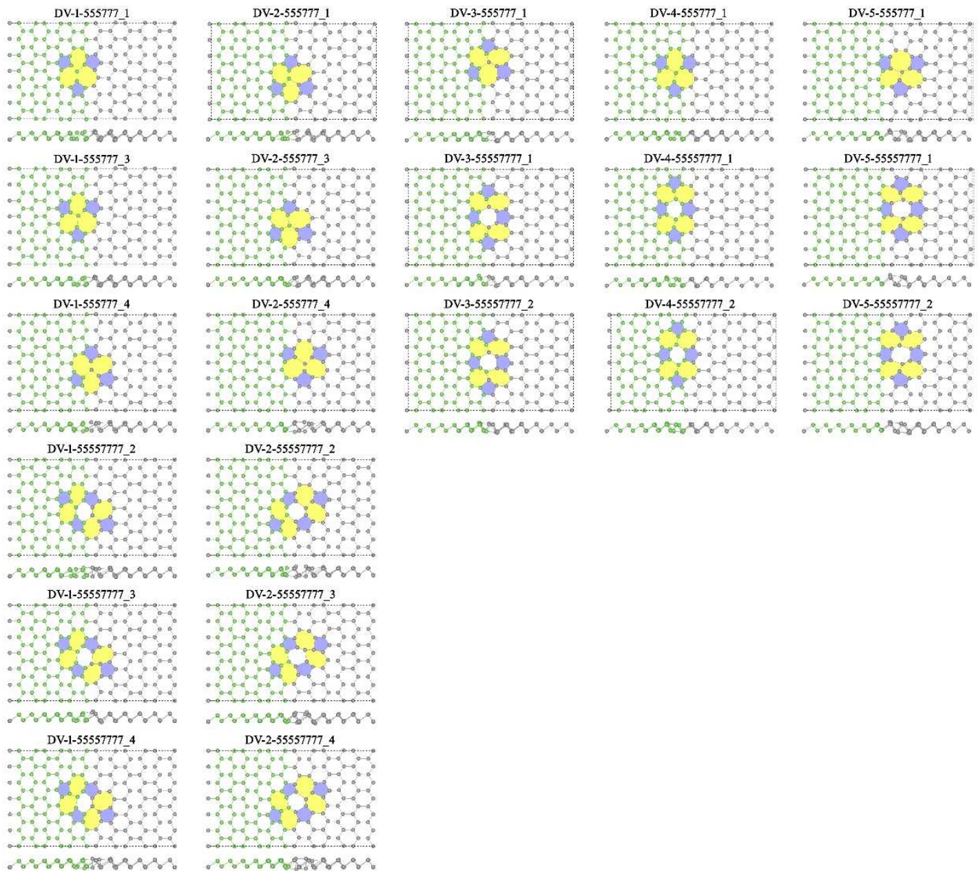
Fig. S2 Top (up) and side (down) views of the optimized structures of interface DVs in each group. The pentagon, heptagon, and octagon are colored in blue, yellow, and green, respectively. The As and Sb atoms are represented by the green and gray balls, respectively.
