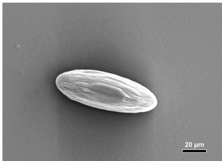
**Figure S8.** SEM image of a nanoellipsoids-based supraparticle dried in the presence of an external magnetic field of 470 Oe.
