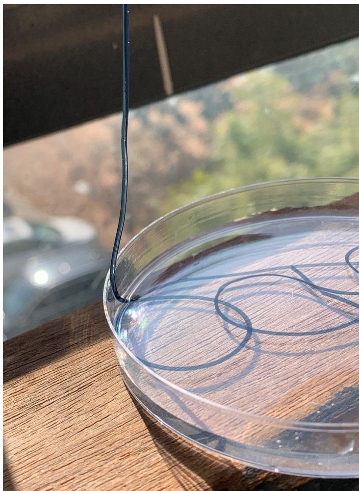
Fig. S1 Digital photo of as-spun PEDOT: PSS/SA composite ( x=1:3 ) fibers via wet-spinning.
