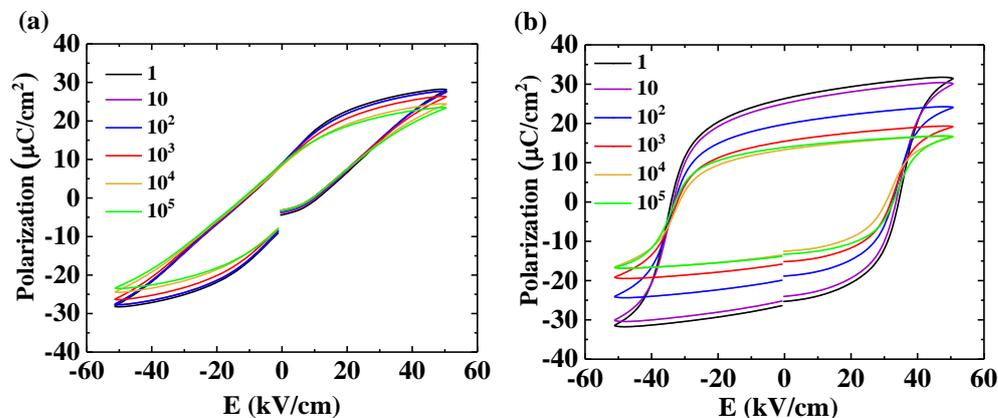
Fig. S3 Evolution of P(E) loops of NBT-BT-3KNN (at 40 °C) and NBT-12BT (at room temperature) fatigued at 50 kV/cm up to  $10^5$  cycles.
