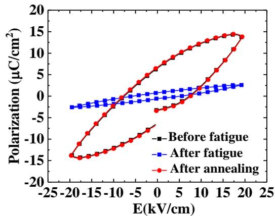
Fig. S4 P(E) loops of NBT-6BT before, after fatigue at 19 kV/cm till  $10^5$  cycles and after annealing treatment.
