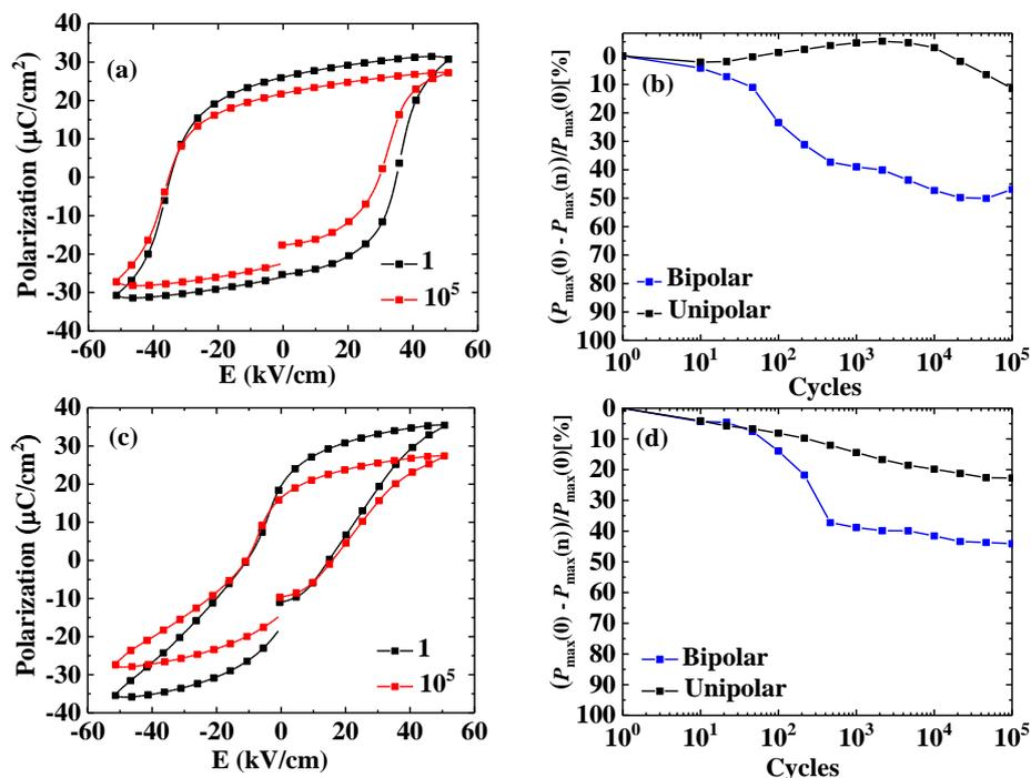
Fig. S2 (a),(c) P(E) loops for unipolar fatigue at room temperature and (b), (d) Comparison of evolution of  $P_{\max}$  for unipolar and bipolar fatigue experiments for NBT-12BT, NBT-BT-3KNN respectively.
