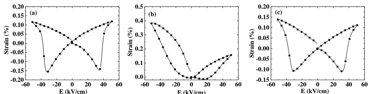
Fig. S1  $S(E)$  loops of NBT-6BT (at room temperature), NBT-BT-3KNN (at 40 °C), NBT-12BT (at room temperature).
