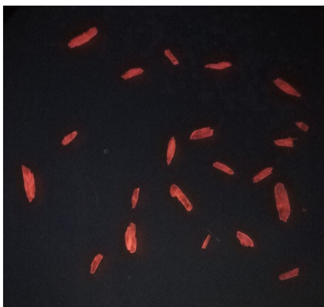
Figure S8. Photography of red luminescent IAM19-1b (Eu 3+ , Ce 3+ -MOF) obtained from single crystal after PSTM under irradiation at 254 nm with a 4 W hand-held UV lamp.
