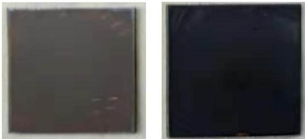
**Figure S1.** a) Variation in color of perovskite precursors with different incorporating ratios of F4TCNQ. b) Perovskite films spin-coated from control and 5 Vol. % precursors.
