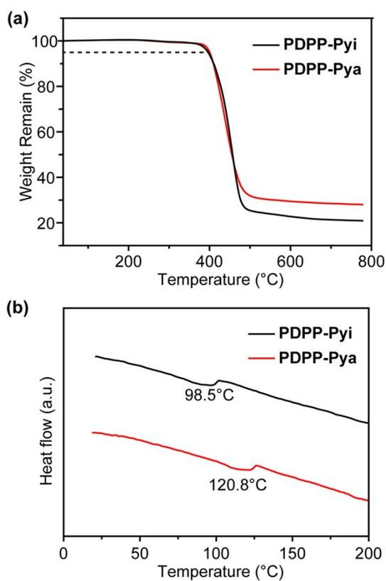
**Fig. S7.** TGA (a) and DSC curves (b) of **PDPP-Pyi** and **PDPP-Pya**.
