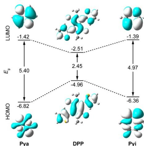
**Fig. S10.** DFT-calculated HOMO, LUMO, bandgap ( $E_g$ ), and frontier orbital distributions of the comonomers of **Pya**, **DPP** and **Pyi** (the isosurface value is 0.02).
