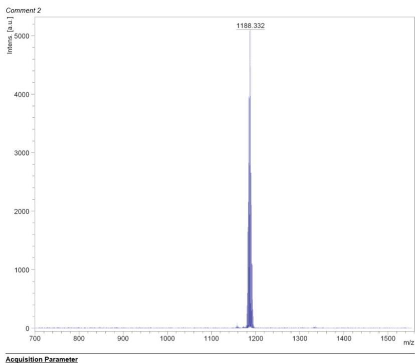
**Fig. S3** MALDI-TOF MS spectrum of **DPP-Sn**.
