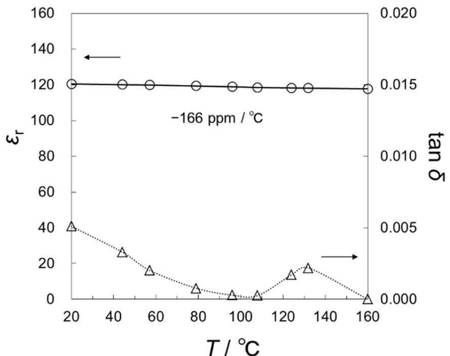
**Fig. S2** Temperature dependence of the dielectric constant  $\epsilon_r$ , and loss  $\tan \delta$  values determined for  $(\text{Bi}_{1-x}\text{Ga}_x)_{2-d}\text{Ti}_2\text{O}_{7-3d/2}$  (sample 29 ( $x = 0.06$ ,  $d = 0.15$ )) at 1 MHz.
