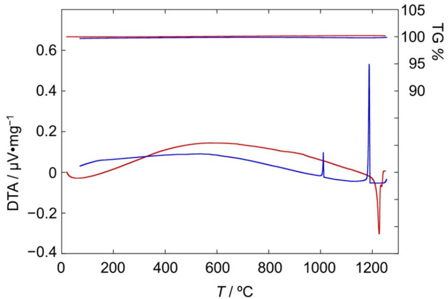
**Fig. S1** TG-DTA curves generated by  $(\text{Bi}_{1-x}\text{Ga}_x)_{2-d}\text{Ti}_2\text{O}_{7-3d/2}$  ( $x = 0.09$ ,  $d = 0.08$ , sample 35) on heating (red) and on cooling (blue).
