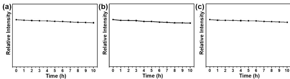
**Fig. S3.** Photostability of B- (a), G- (b), and R-CDs (c) under continuous illumination with an UV (365 nm, 5 W) lamp for 10 h.
