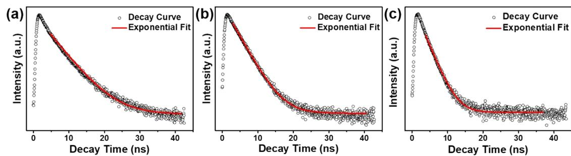
**Fig. S2.** Time-resolved PL spectra of B- (a), G- (b), and R-CDs (c), respectively.
