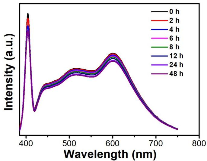
**Fig. S6.** EL spectra of the WLED recorded under different operating time intervals.
