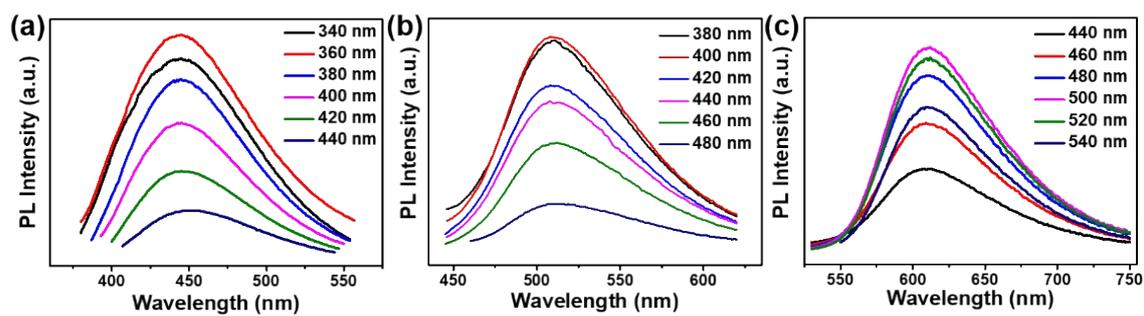
**Fig. S1.** PL spectra of B- (a), G- (b), and R-CDs (c) recorded upon excitation at different wavelengths.
