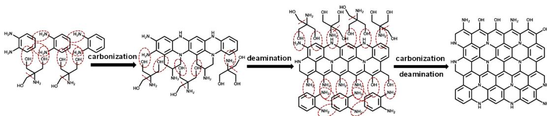
**Fig. S4.** Illustration of the growth mechanism of Tri-CDs.
