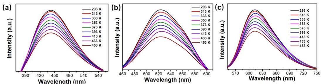
**Fig. S5.** PL spectra of B-, G- and R-CD films (left to right) at different temperatures from 293 to 453 K.
