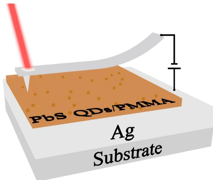
Figure S6. Schematic diagram of CAFM measurement. According to the Guidebook of CAFM, the test base is the positive electrode.
