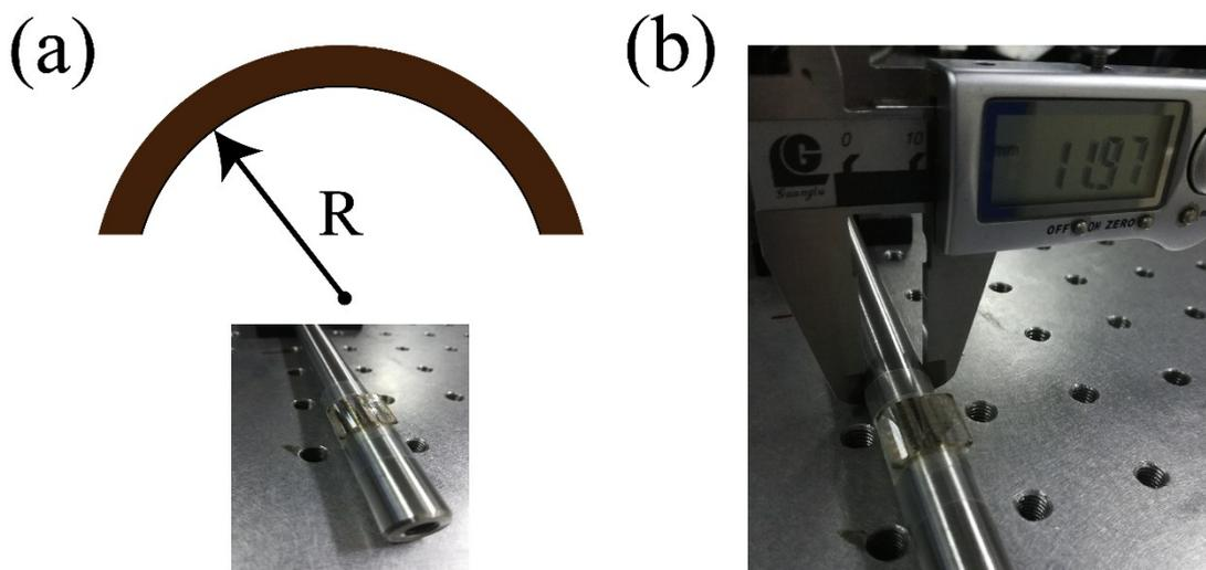
Figure S4. Schematic diagram of bending test.
