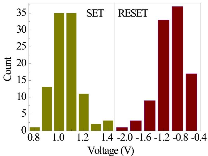
Figure S3. Statistical distribution of the  $V_{SET}$  and  $V_{RESET}$ . The results are obtained from I-V sweep mode of 100 cycles.
