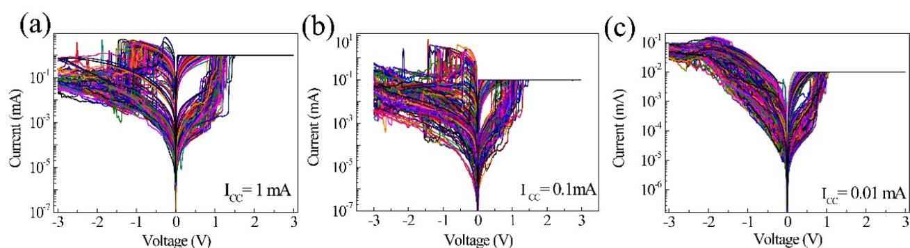
Figure S2. I-V curves of 100 cycle sweeps in different compliance currents of the device.
