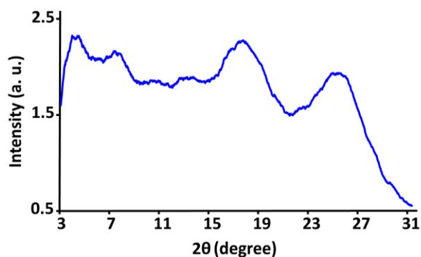
**Fig. S4** XRD pattern of amorphous pristine PEDOT:PSS film showing some degree of crystallinity.
