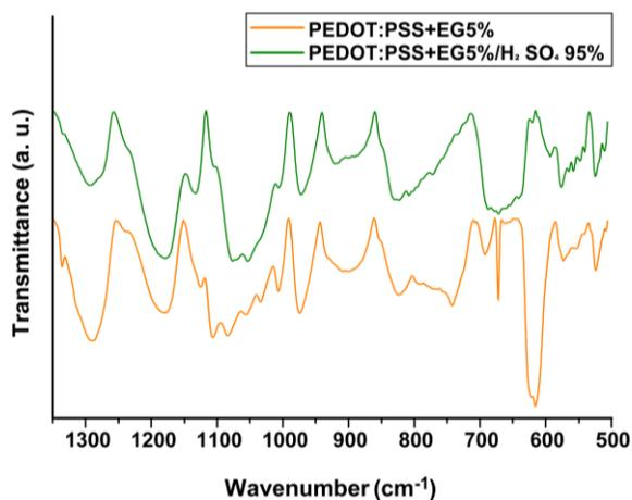
**Fig. S2** Transmission FTIR spectra of EG-doped, and sulfuric acid post-treated PEDOT:PSS thin films. The spectra are similar to the DMSO-doped samples.
