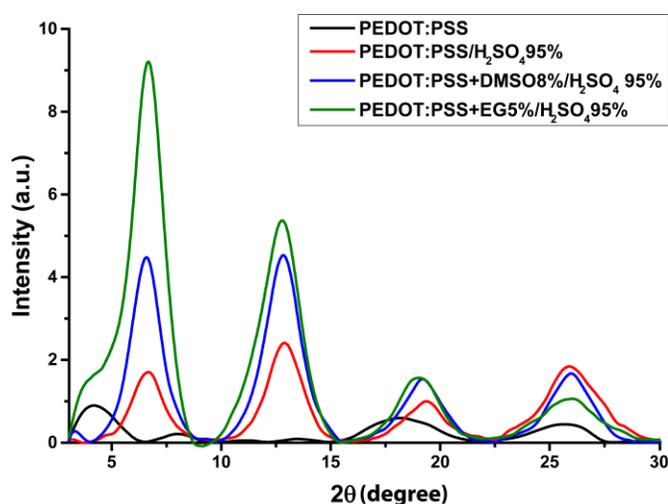
**Fig. S5** XRD diffractograms of pristine, solvent-doped, acid post-treated and solvent-doped/acid post-treated PEDOT:PSS films.
