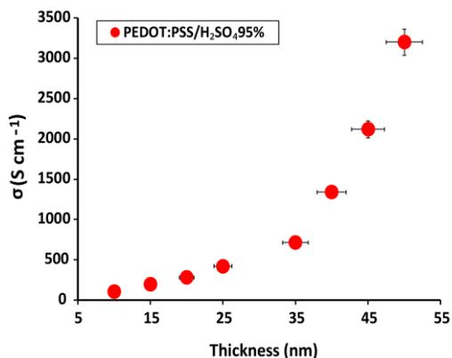
**Fig. S1** Conductivity correlation with thickness in PEDOT:PSS thin films treated with H<sub>2</sub>SO<sub>4</sub> 95%.
