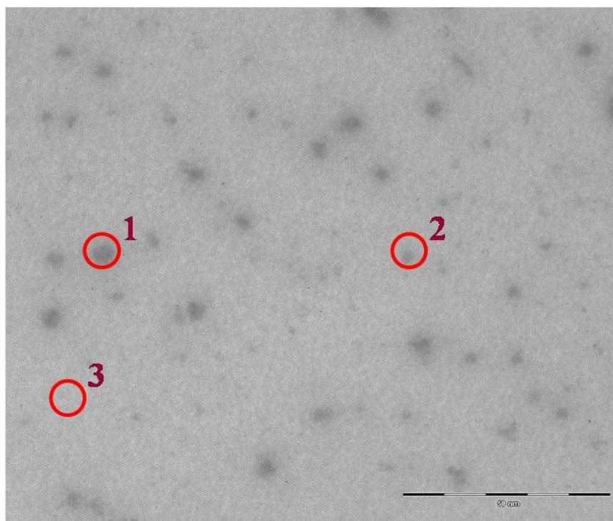
**Figure S3.** TEM image of  $\text{Sn}_{0.92}\text{Bi}_{0.04}\text{Zn}_{0.04}\text{Te}$  revealing  $\text{Zn}$  nanoprecipitates. The scale bar represents 50 nm. The percentage elemental compositions of the area marked in red circles are given in Table S2.
