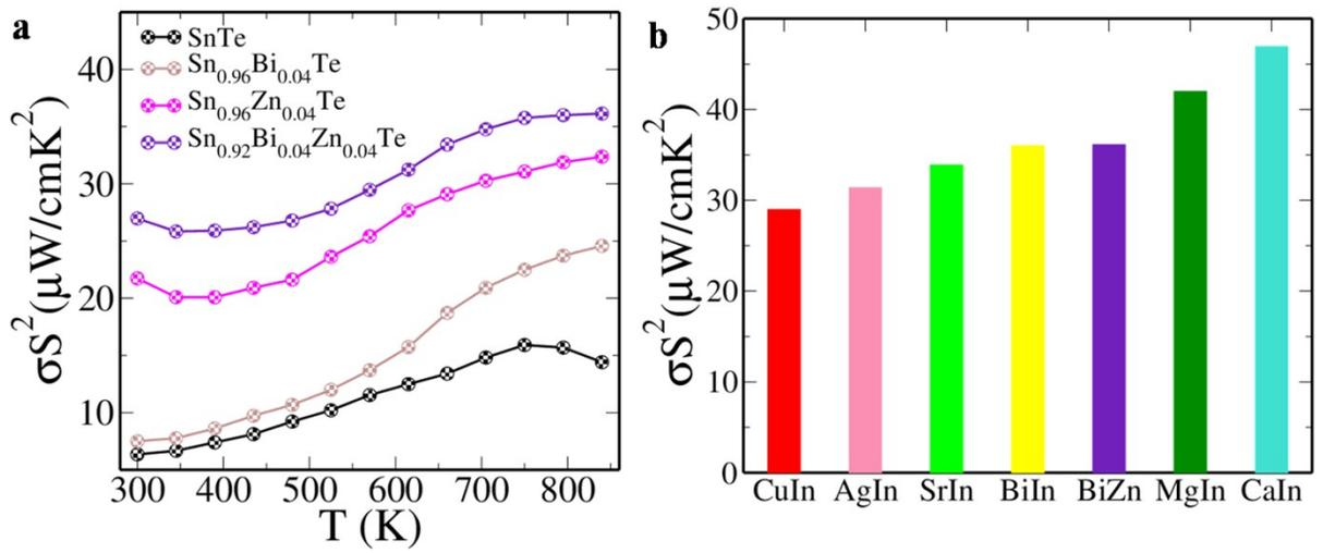
**Figure S4.** a) Power factor as a function of temperature for pristine SnTe and doped samples; b) Comparison of power factor of  $\text{Sn}_{0.92}\text{Bi}_{0.04}\text{Zn}_{0.04}\text{Te}$  with state of the art SnTe based materials with high power factor.<sup>1-6</sup>
