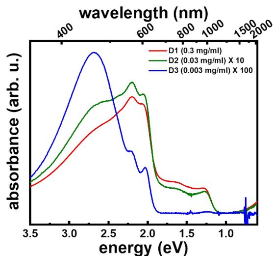
Figure S7: Effect of dilution of BCF doped RRe-P3HT (1:4) starting from an absolute concentration of 3 mg/ml. In all cases the absorption features of the polaron in aggregated P3HT as well as neutral aggregated P3HT are present. This indicates the stability of the aggregates (both neutral and doped) is enhanced with the presence of dopant.
