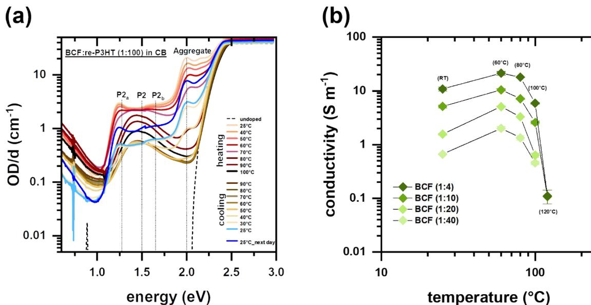
Figure S3: Temperature dependence of (a) Optical absorption spectra of BCF:re-P3HT (1:100) in chlorobenzene solution and (b) electrical conductivity of BCF:re-P3HT thin films at different dopant
