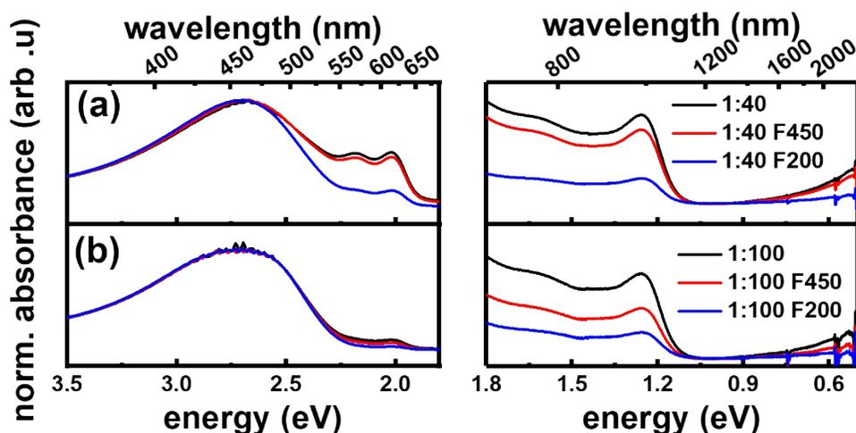
Figure S5: Changes of optical absorption spectra of BCF doped P3HT suspensions with filtration for absolute concentration of 1 mg/ml for (a) dopant ratio of 1:40 and (b) 1:100.
