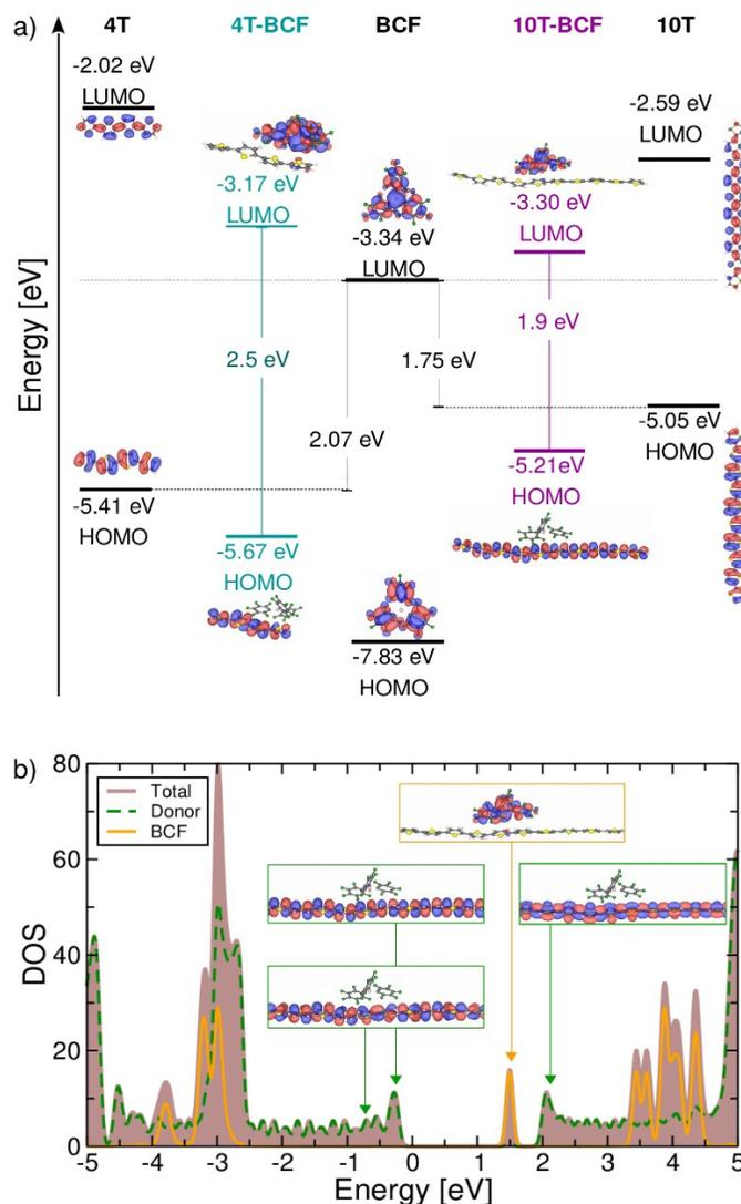
Figure S2: a) Energies and spatial distribution of the frontier orbitals of BCF with respect to the considered thiophene oligomers and the resulting D/A complexes computed from density functional theory. b) Density of states (DOS) representing the total as well as the donor and acceptor contributions of BCF-doped polythiophene. The spatial distribution of selected states close to the frontier are shown in the inset.
