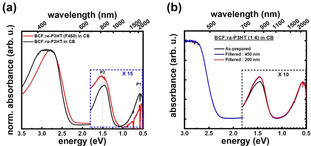
Figure S4: Optical absorption spectra of BCF:P3HT (1:4) in (a) doped single chains in solution of *ra*-P3HT (black) and filtered *re*-P3HT suspension (red) – inset is a zoom into the absorption features of the polarons – and (b) optical absorption spectra of BCF:*ra*-P3HT (1:4) before and after filtration with F450 and F200. *Ra*-P3HT solution is prepared at the absolute concentration of 2 mg/ml.
