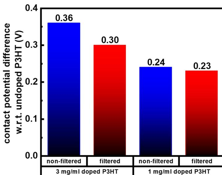
Figure S8: Contact potential difference with reference to undoped P3HT (0V) in thin films of P3HT spin-coated from filtered and non-filter suspensions at two different dopant concentrations. All data are for doped films with 1:4 dopant ratio.
