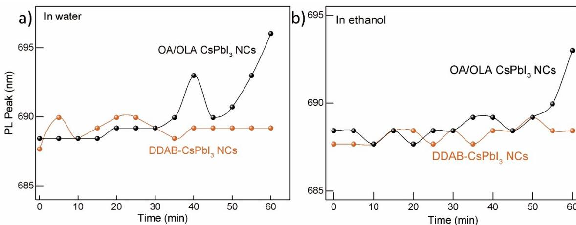
**Figure S5** The PL peak of OA&OLA CsPbI<sub>3</sub> NCs and DDAB-capped CsPbI<sub>3</sub> NCs in **a)** water and **b)** in ethanol as a function of time.
