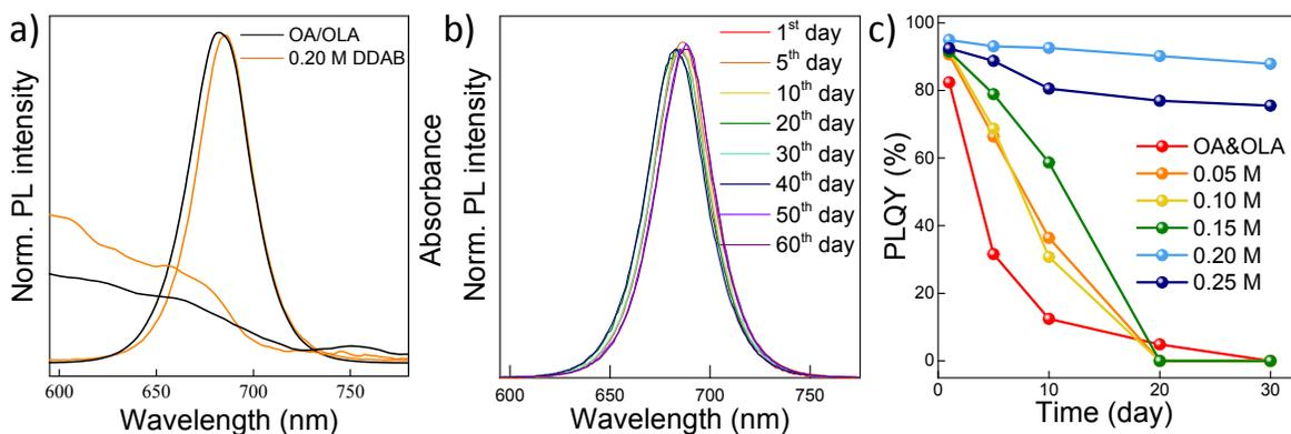
**Figure S1** a) Room temperature PL and absorbance spectra of OA/OLA and DDAB-capped perovskite nanocrystals measured on the 1<sup>st</sup> day after synthesis. b) Room temperature PL of DDAB-capped NCs measured over 60-day period. c) The PLQY of perovskite nanocrystals prepared with OA/OLA and different concentrations of DDAB as a function of time.
