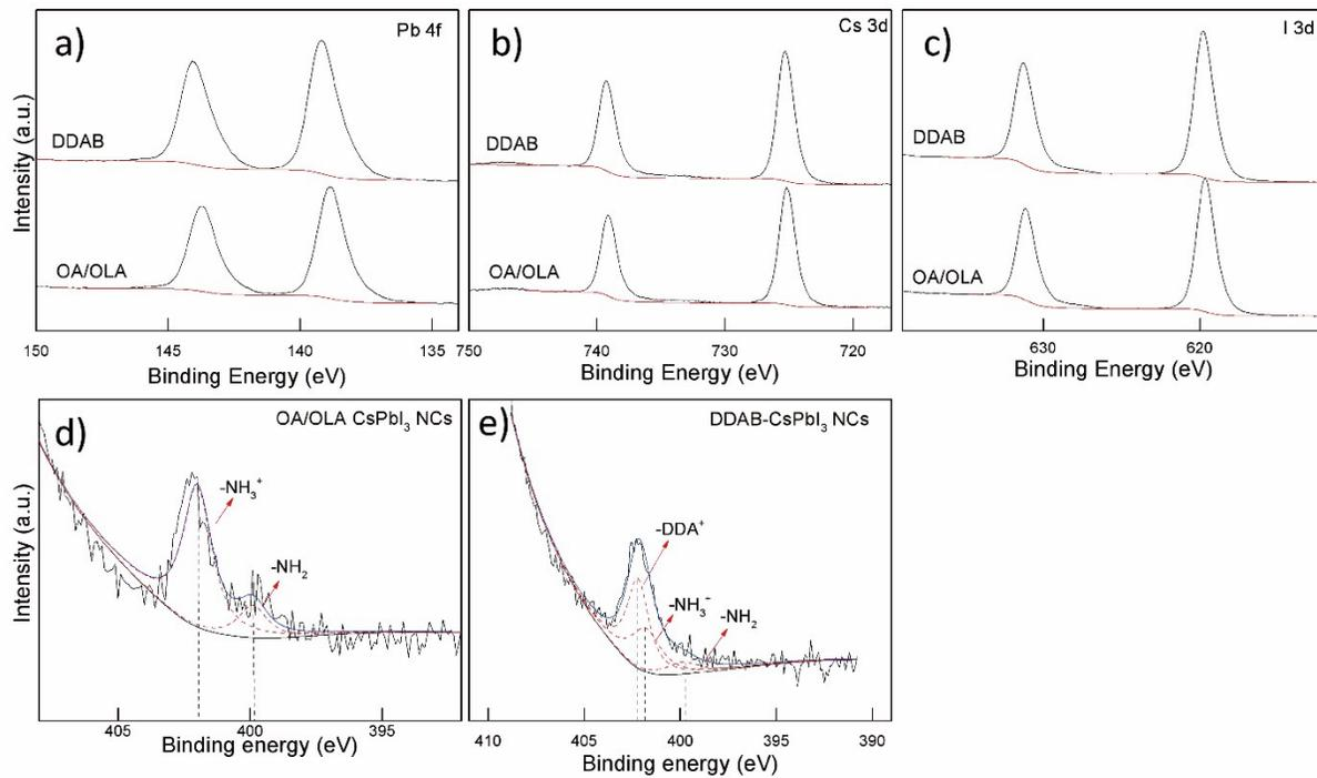
**Figure S4** XPS spectra of **a)** Cs 3d, **b)** Pb 4f, **c)** I 3d, **(d-e)** N1s of OA&OLA CsPbI<sub>3</sub> NCs and DDAB-capped CsPbI<sub>3</sub> NCs.
