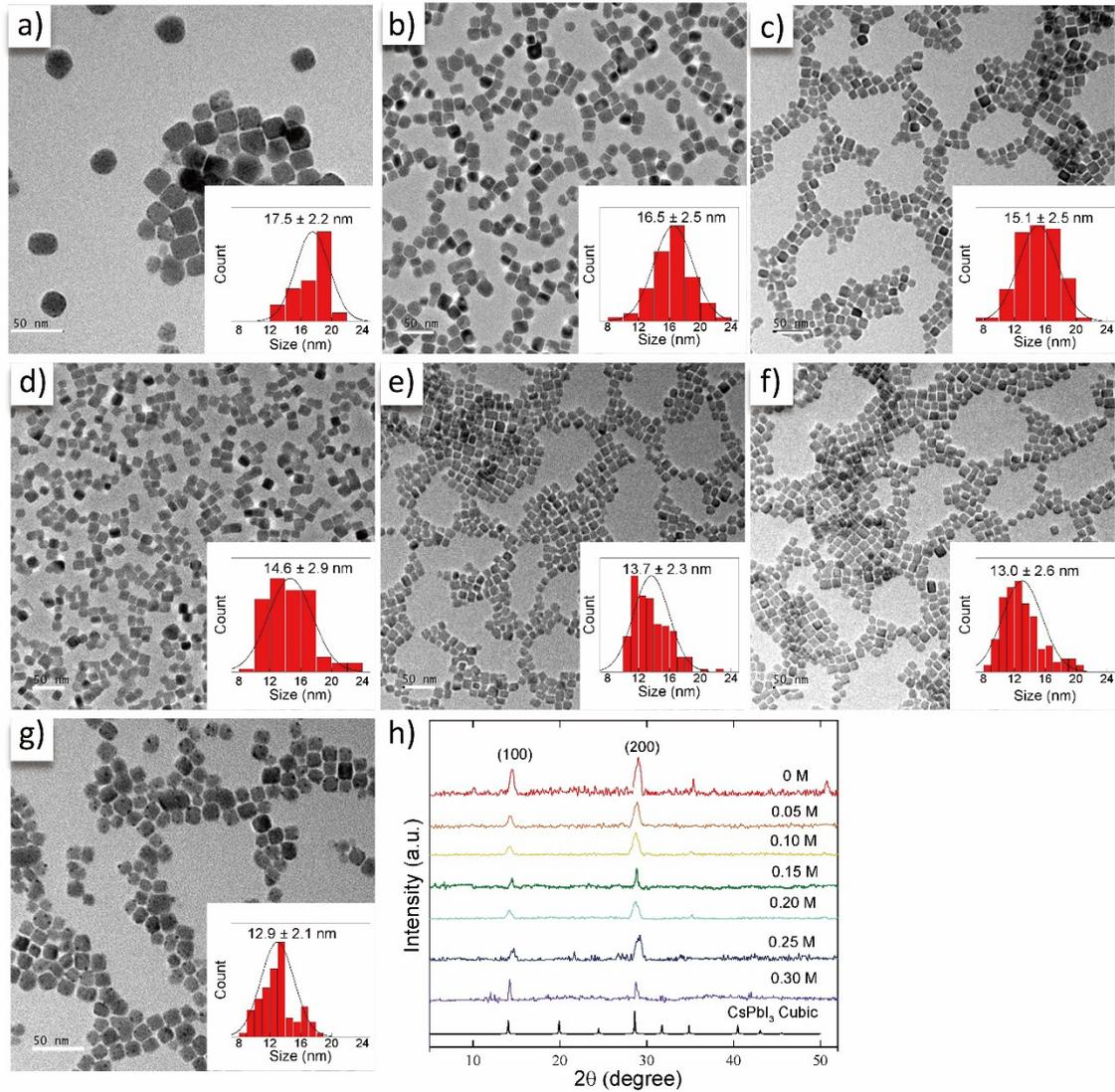
**Figure S2** TEM images of CsPbI<sub>3</sub> NCs prepared with different concentrations of DDAB **a)** 0 M, **b)** 0.05 M, **c)** 0.10 M, **d)** 0.15 M, **e)** 0.20 M, **f)** 0.25 M, **g)** 0.30 M. **h)** XRD patterns of CsPbI<sub>3</sub> NCs films obtained by different concentration of DDAB.
