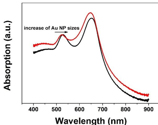
**Fig. S5** The extinction spectra of the *hncp* Au NP arrays with different Au NP sizes (red line of 190 nm and black line of 260 nm in diameter of Au nanoparticles).
