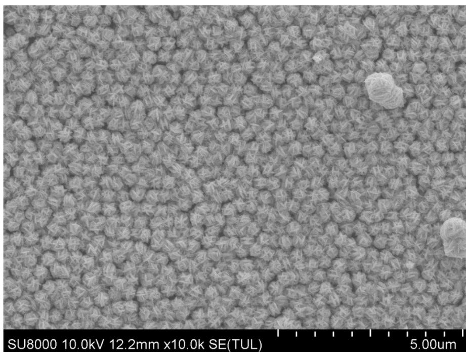
**Fig. S8** SEM image of the hexagonally patterned flower-shaped Au@Ag NP arrays with the periodicity of 350 nm.
