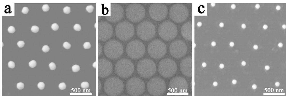
**Fig. S1** SEM images of nanoparticle (NP) arrays as the growth template: (a) the hexagonal non-close-packed (*hncp*) Au NP arrays. (b) the *hncp* polystyrene (PS) colloidal microsphere arrays. (c) the *hncp* Cu NP arrays.
