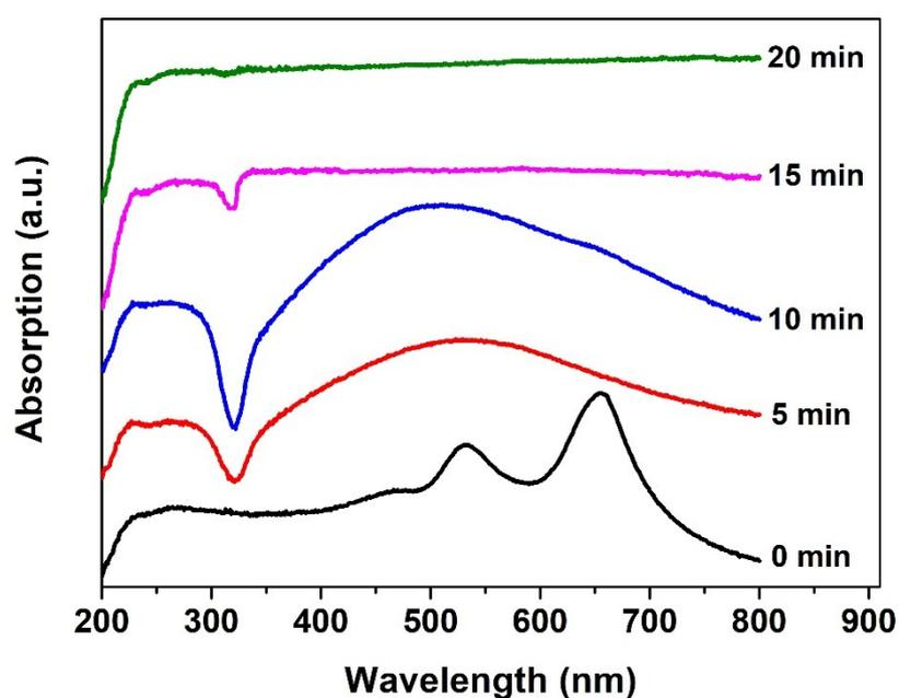
**Fig. S4** The extinction spectra of the *hncp* Au NP arrays (0 min) and the hexagonally patterned flower-shaped Au@Ag NP arrays with different growth time (5-20 min).
