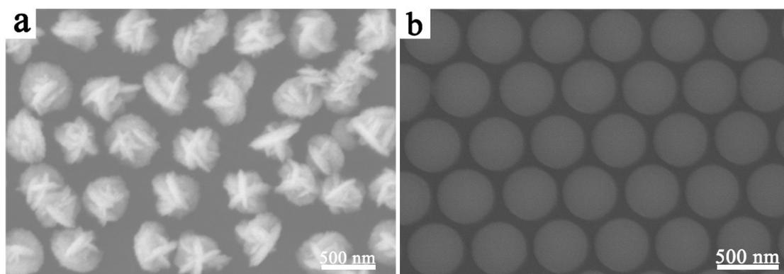
**Fig. S2** (a) SEM image of the flower-shaped Cu@Ag NP arrays using *hncp* Cu NP arrays as the growth template. (b) SEM image of the obtained array without Ag nanosheets grown on it using hexagonally patterned PS colloidal microsphere arrays as the growth template.
