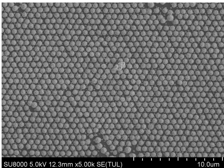
**Fig. S9** SEM image of the hexagonally patterned flower-shaped Au@Ag NP arrays with the periodicity of 750 nm.
