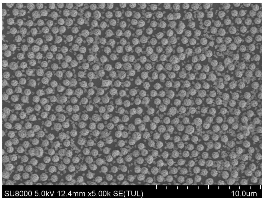
**Fig. S10** SEM image of the hexagonally patterned flower-shaped Au@Ag NP arrays with the periodicity of 1000 nm.
