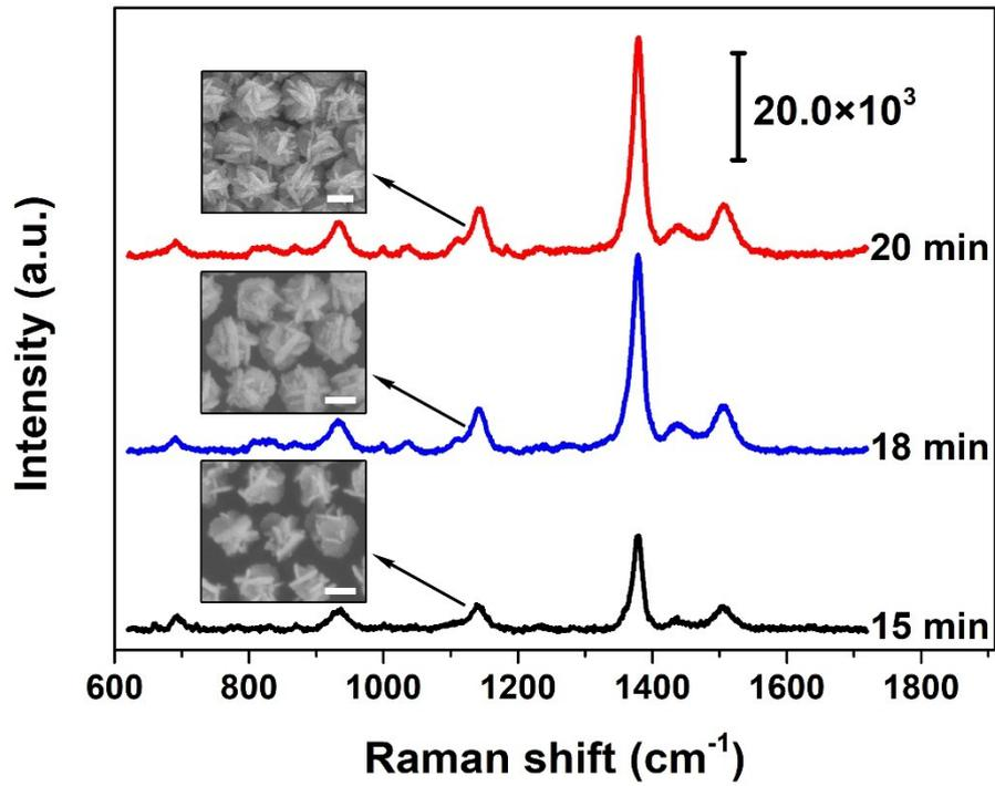
**Fig. S11** Raman spectra of  $10^{-7}$  M thiram on the hexagonally patterned flower-shaped Au@Ag NP arrays (350 nm in periodicity) with different growth time (15, 18 and 20 min). Insets: corresponding SEM images. Scale bars in insets: 200 nm.
