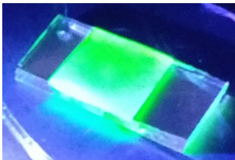
**Fig. S1.** The fluoresce image of the sequentially evaporated cesium lead bromide film (with an effective area about 1.2 cm × 1.2 cm) taken under the illumination of 375 nm UV light.
