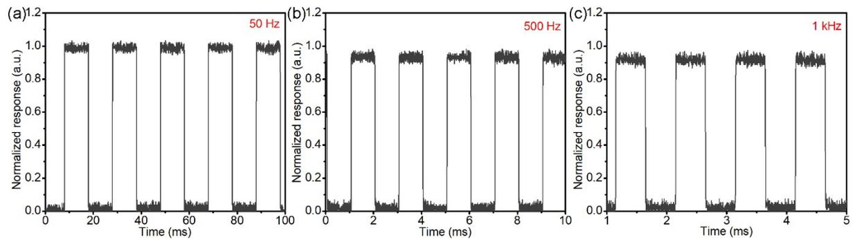
**Fig. S5.** Photoresponse of the PMMA-modified device recorded under 450 nm illumination at varied frequencies of (a) 50 Hz, (b) 500 Hz and (c) 1 kHz.
