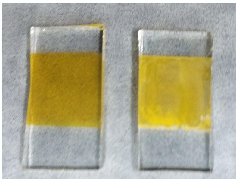
**Fig. S2.** Camera image of the CsPbBr<sub>3</sub> films prepared via sequential evaporation (left) and traditionally two-step solution method (right).
