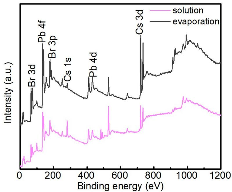
**Fig. S3.** XPS survey of the conventionally solution-processed and evaporated CsPbBr<sub>3</sub> films.
