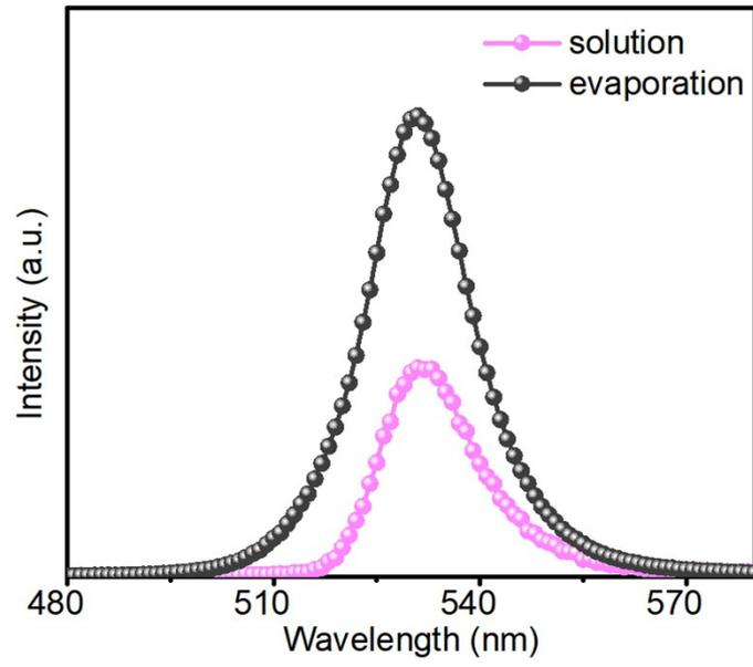
**Fig. S4.** Steady-state PL of the solution-processed and evaporated CsPbBr<sub>3</sub> films deposited on ITO substrates.
