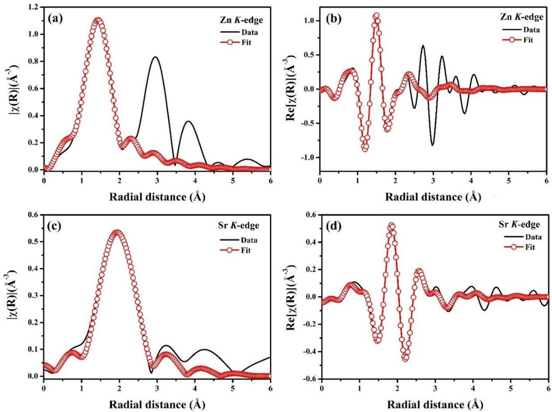
**Figure S2:** (a) and (c) represents magnitude of Fourier transformed EXAFS function for Zn K-edge and Sr K-edge, respectively. (b) and (d) represents real part of Fourier transformed EXAFS function for Zn K-edge and Sr K-edge, respectively. (The Fourier transformed curves shown here are phase uncorrected).
