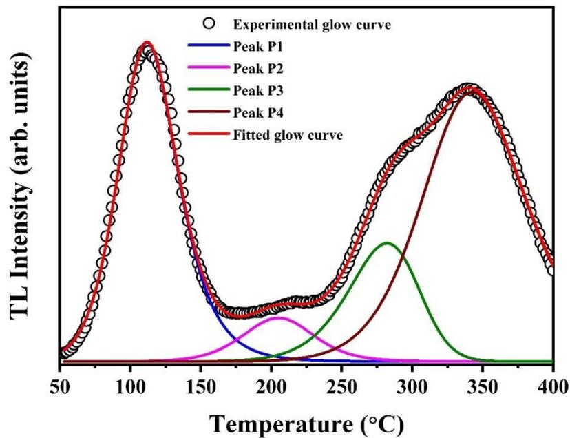
**Figure S3:** Computerized glow curve deconvolution of thermoluminescence glow curve obtained at 1 kGy gamma radiation dose.
