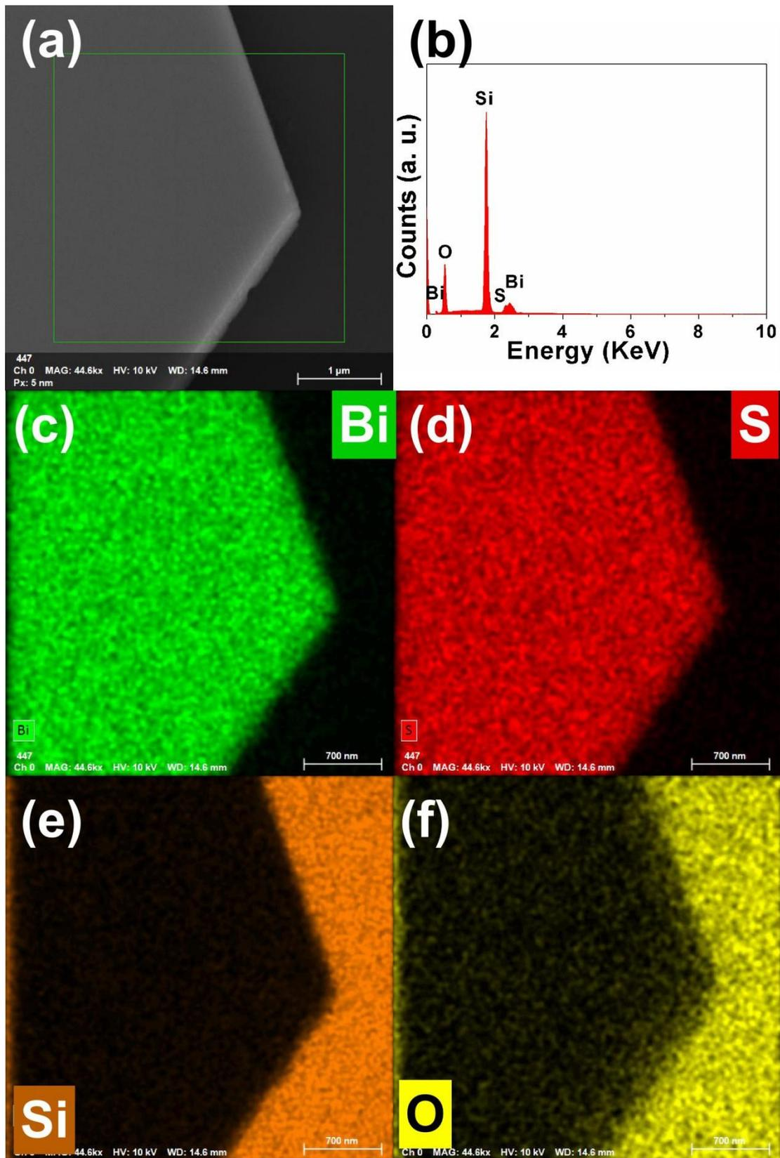
**Fig. S1** a) SEM image of the edge of a  $\text{Bi}_2\text{S}_3$  nanobelt. b) EDS spectra of a  $\text{Bi}_2\text{S}_3$  nanobelt. c)-f) Corresponding individual elementary distribution of Bi, S, Si and O.
