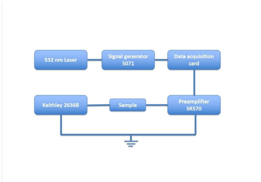
**Fig. S2** Schematic illustration of the layout of self-designed photoresponse testing system for  $\text{Bi}_2\text{S}_3$  nanobelts.
