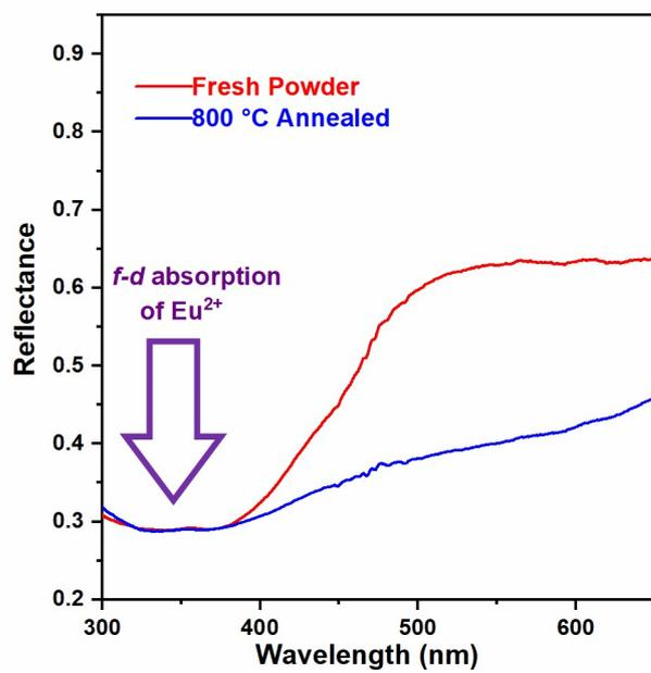
**Figure S6.** Reflectance spectra of SrSi<sub>2</sub>O<sub>2</sub>N<sub>2</sub>:1%Eu before and after annealing.
