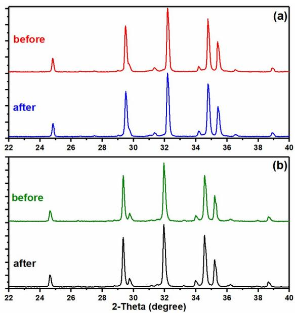
**Figure S7.** XRD patterns of (a) SrLuAl<sub>2</sub>Si<sub>2</sub>O<sub>2</sub>N<sub>5</sub> and (b) BaLuAl<sub>2</sub>Si<sub>2</sub>O<sub>2</sub>N<sub>5</sub> before and after water immersion before and after 5 days water immersion.
