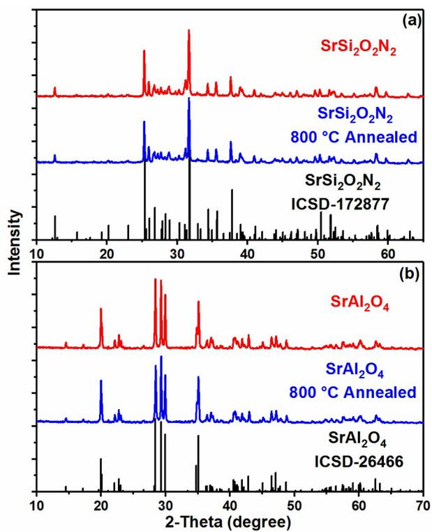
**Figure S4.** XRD profiles of (a)  $\text{SrSi}_2\text{O}_2\text{N}_2$  and (b)  $\text{SrAl}_2\text{O}_4$  before and after annealing treatment at  $800\text{ }^\circ\text{C}$ . ( $\text{SrAl}_2\text{O}_4$  was selected to represent the oxide hosts)
