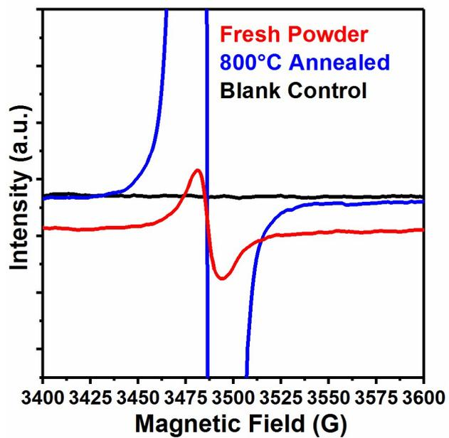
**Figure S5** ESR spectra of  $\text{SrSi}_2\text{O}_2\text{N}_2:1\%\text{Eu}$  before and after annealing (focus in the range of 3400-3600 G).
