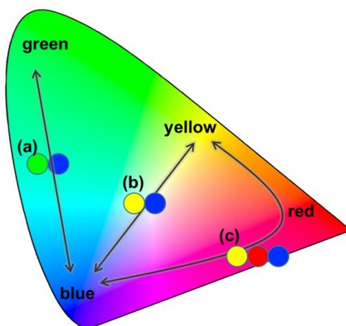
**Fig. S1** Chromaticity diagram to indicate the color variation ranges of (a) green- and blue-emission, (b) yellow- and blue-emission, and (c) yellow-, red- and blue-emission based fluorescence sensors.
