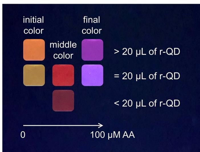
**Fig. S6** Fluorescence colors of MnO<sub>2</sub>-OPD-QDs sensors containing different volumes of r-QDs before and after interaction with AA.
