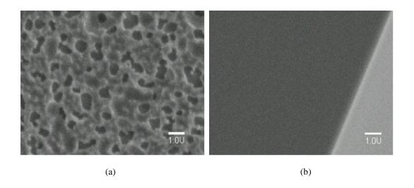
**Fig. SI2** SEM of the surface features of n<sup>+</sup> type germanium after (a) 2 min and (b) 5 min anodization under 350 mA/cm<sup>2</sup>. Oxide layer formed during first 2 min of anodization dissolved during next 3 min of anodization. Diagonally fractured top surface was included in (b) in order to compare the cleanliness of the top surface.
