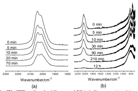
**Fig. SI1** FTIR studies of stability tests of PG in boiling water (a) and in oven at 100 °C (b).
