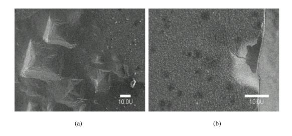
$\textbf{Fig. SI3} \hspace{0.2cm} \textbf{SEM (plan view) of } n^{^{+}} \hspace{0.2cm} \textbf{type PG.} \hspace{0.2cm} \textbf{Pyramidal shape surface features (a) and nanoparticles (b) are shown.}$
