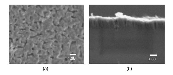
Fig. SI5 Plan and cross-sectional view of (a and (b) p type derived PG.
