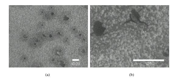
**Fig. SI4** SEM of the plan view of p type PG. Submicron-sized particles were found around the edge of the sample. Fractured areas and nanoparticles are seen under lower (a) and higher magnification (b).
