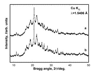
Fig. 2. The x-ray powder diffraction patterns of phenacyltriphenylphosphonium bromide 1 prepared mechanochemically by ball-milling of triphenylphosphine and 2-bromoacetophenone for one hour without solvent (a), and commercial bromide 1 (Lancaster Synthesis) ball-milled for one hour (b).
