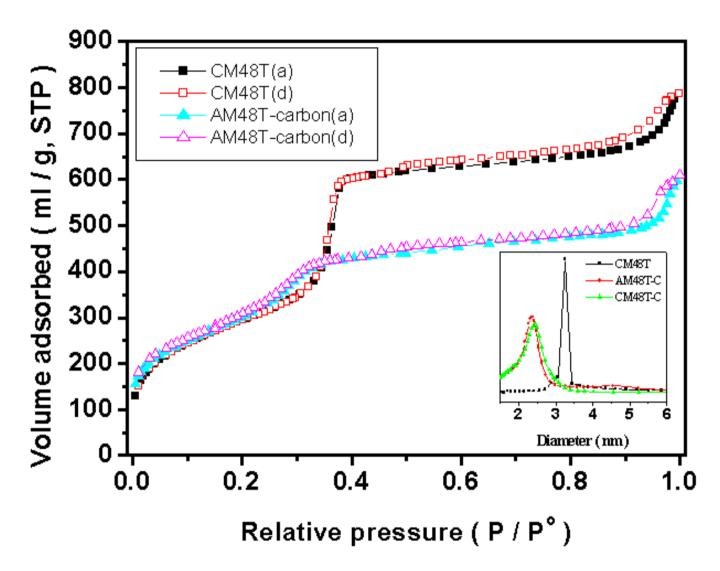
$\rm N_2$  adsorption and desorption isotherms of the CM48T and the AM48T-carbon replica. The Insert provides the corresponding pore size distribution curves calculated from the adsorption branch of the nitrogen isotherm by the BJH method. The isotherms were measured at 77 K on a Micromeritics ASAP 2000 Gas Adsorption Analyzer after the silica template and carbons were degassed at 423 K to 20  $\,\mu Torr$  for 4  $\sim$  6 h.
