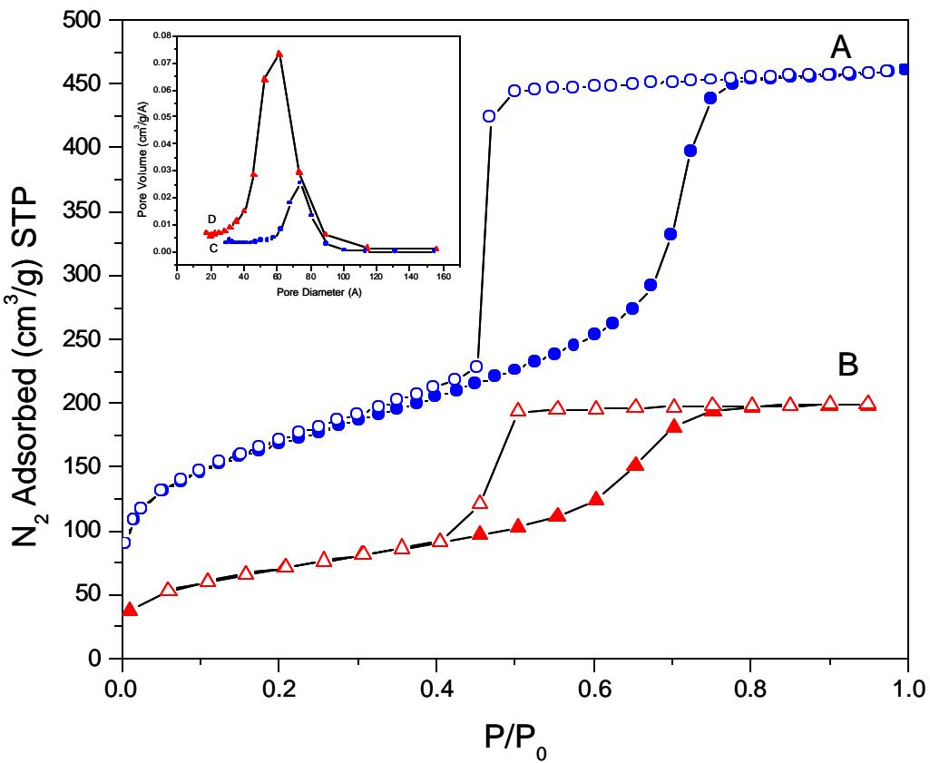
**Figure Caption:** Nitrogen adsorption and desorption isotherms for (A) control blank mesoporous silica and (B) U<sub>3</sub>O<sub>8</sub>-incorporated mesoporous silica. Insert: pore distribution of (C) control blank mesoporous silica and (D) U<sub>3</sub>O<sub>8</sub>-incorporated mesoporous silica. The surface areas of control blank sample and U<sub>3</sub>O<sub>8</sub>-incorporated mesoporous sample are 568.2 m<sup>2</sup>/g and 250 m<sup>2</sup> g<sup>-1</sup>, respectively.
