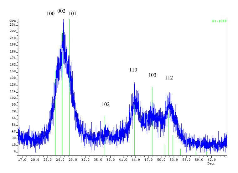
Peak assignments based on wurtzite mineral (greenockite, jps card 41-1049)Cu K-alpha radiation.
