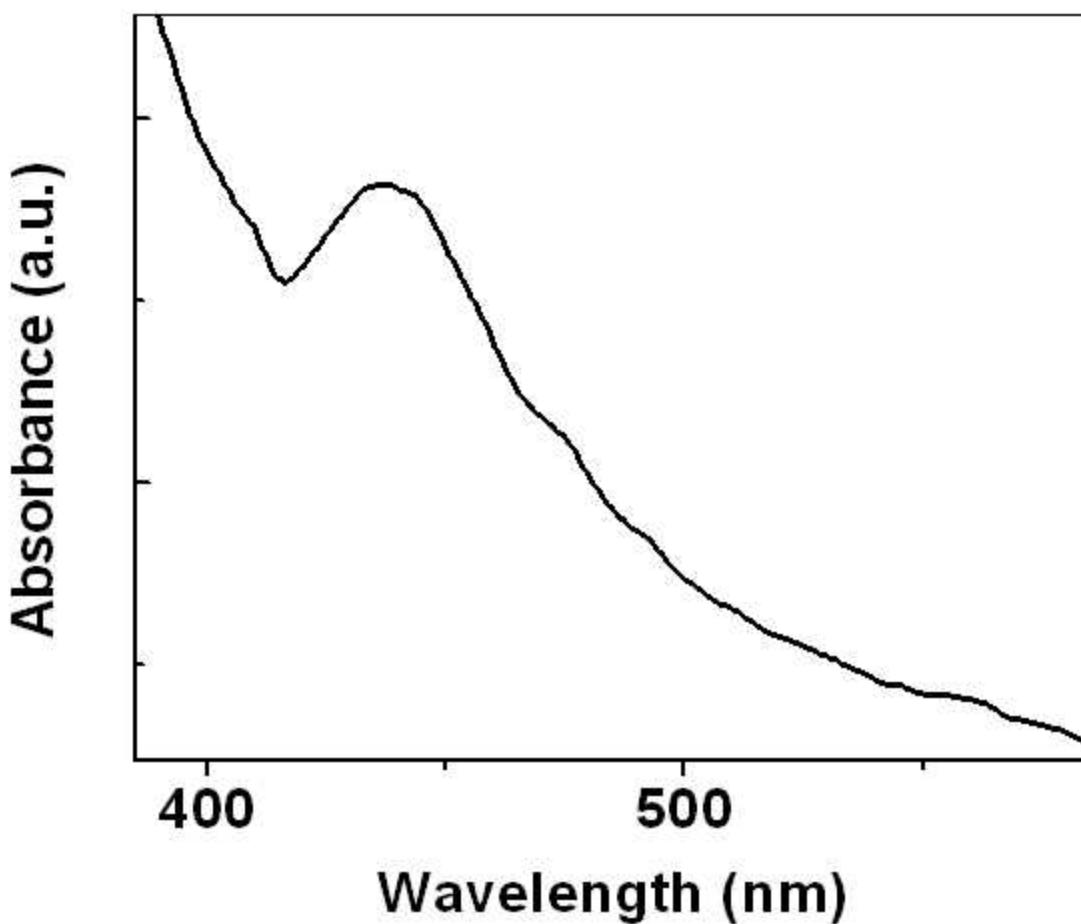
S1. UV-vis absorption spectrum of gold nanosheets grown using anthracene anions at the liquid-liquid interface.
