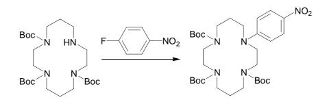
A solution of 1-fluoro-4-nitrobenzene (0.212 mL, 2 mmol) in toluene (25 mL) was added dropwise to a boiling solution of 1,4,8-Tris(*tert*-butoxycarbonyl)-1,4,8,11-tetraazacyclotetradecane (0.5g, 1 mmol) and triethylamine (0.278 mL, 2 mmol) in toluene (75 mL). The solution was maintained under reflux for 24 hrs. The solvent and the excess of triethylamine were removed in vacuo and the residue was purified by liquid chromatography (silica gel, ethyl acetate/hexane 2:3, Rf=0.5).
