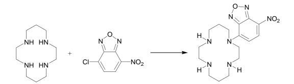
A solution of 4-chloro-7-nitro-benzofurazan in toluene (2 mmol in 40 mL) was added dropwise to a boiling solution of cyclam in toluene (10 mmol in 150 mL). The solution was maintained under reflux for 3 hrs. On cooling, unreacted cyclam precipitated and was separated through filtration. The solution was then concentrated at the rotavapor to give a ruby red precipitate, which was separated through filtration under vacuum and dried under vacuum.
