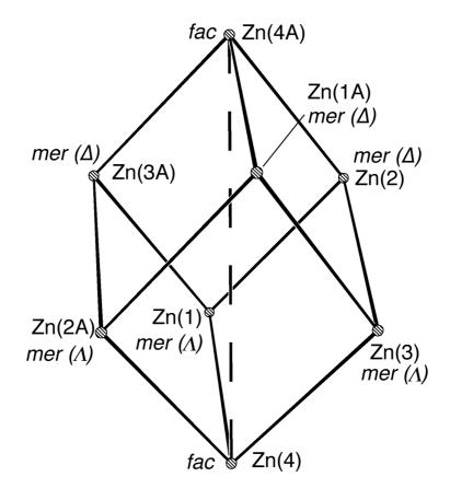
**Figure S1**. A view of the metal polyhedron emphasising the rotational symmetry (the dotted line is the  $C_3/S_6$  axis)
