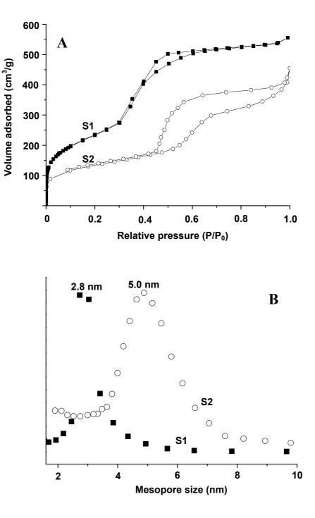
7,  $N_2$  sorption curves (A) and pore size distributions (B) of C1 (templated by MWD-MCM-41) and C2 (templated by leaf-like MCM-41).
