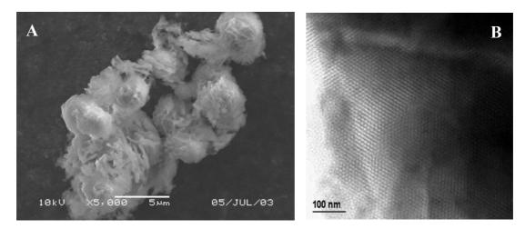
5, FESEM images of carbon nanowire arrays templated by leaf-like MCM-41. Carbon nanotubes can also be observed. It can be observed that the ends of carbon nanowires are covered by thin carbon layers (see enlarged A and B).
