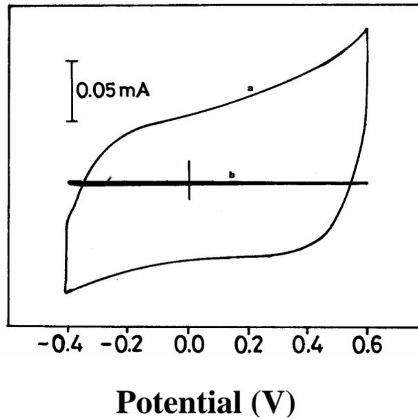
Figure 6. CV of PEDOT/ssDNA in pH 8.0 phosphate buffer at a scan rate of 100 mV/s; a) before exposure to the target ssDNA and b) after exposure to target ssDNA.
