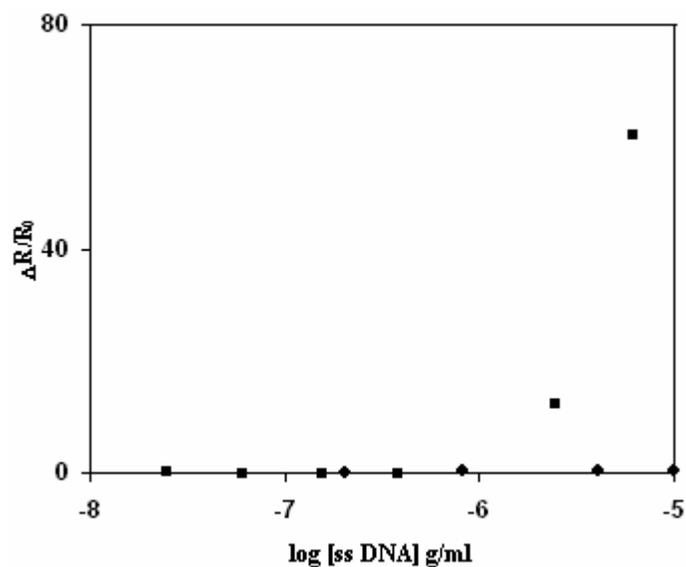
Figure 3. Sensor response using 5mer ssDNA (C1) immobilized PEDOT. ■ sensor response when exposed to a 10mer (B1) with 5mer complementary segment and ● is for a 10mer (B) having 2mer complementary segment.
