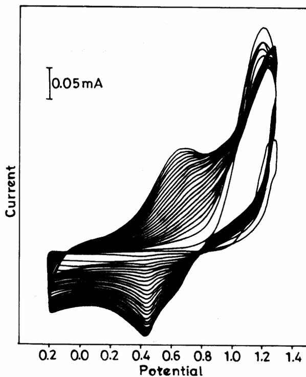
Figure 2. Growth of PEDOT/ss DNA(A) from 0.01M EDOT and 0.1M KCl in pH 8.0 phosphate buffer at a scan rate of 50mV/s.
