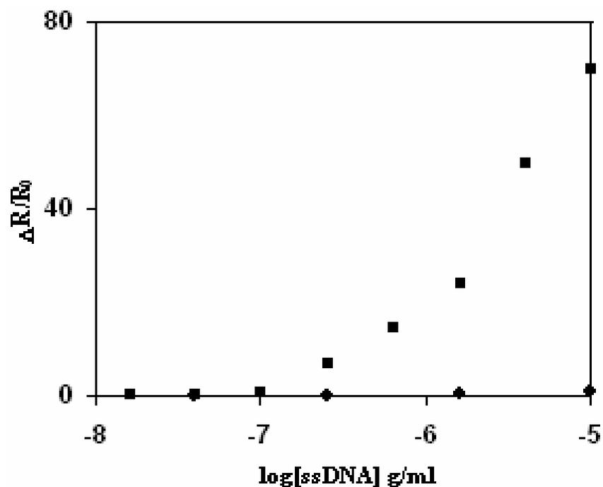
Figure 5. Sensor response using 10mer ssDNA(B) immobilized PEDOT; ■ Sensor response as a function of ssDNA concentration (B1); ● for noncomplementary strand (A).
