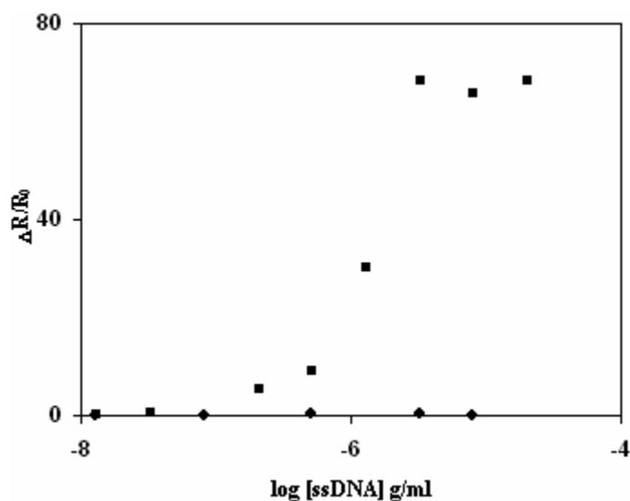
Figure 4. Sensor response using 10mer ssDNA(B) immobilized PEDOT; ■ sensor response when exposed to various concentrations of 5mer (C); ● is for control experiment where the sensing device had no probe ssDNA.
