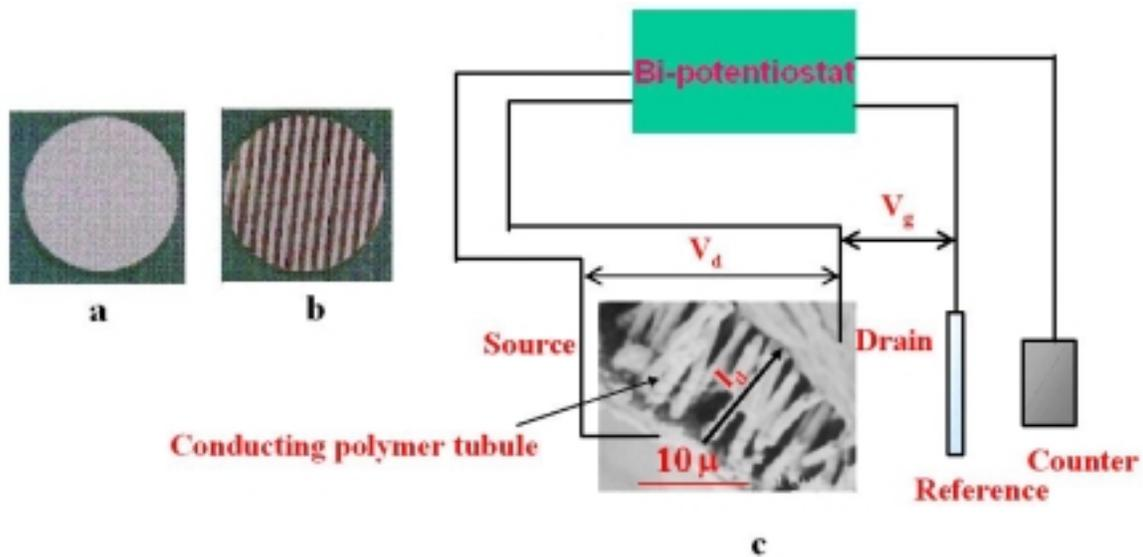
Figure 1: (a) Isoporous polycarbonate membrane, (b) Both side gold coated polycarbonate membrane and (c) Schematic representation of the sensor measurements.
