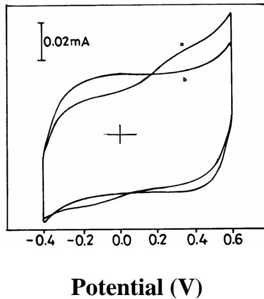
Figure 7. CV of PEDOT (without probe ssDNA) in pH 8.0 phosphate buffer at a scan rate of 100 mV/s; a) before exposure to the ssDNA and b) after exposure to ssDNA.
