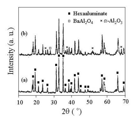
**Fig. 5** XRD patterns of the  $La_{0.95}Ba_{0.05}MnAl_{11}O_{19}$  catalysts prepared in different systems: (a) the novel microemulsion system: Water/PrOH/BuOH=12.5:12.5:75 (vol.%), M(OR)<sub>x</sub>/water=1/100 (mole ratio) (b) pure water
