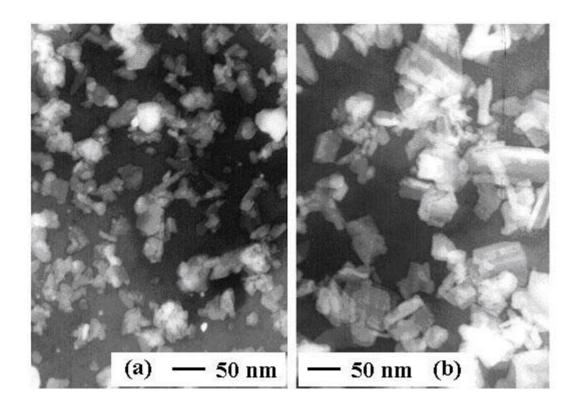
**Fig. 7** TEM images of the  $La_{0.95}Ba_{0.05}MnAl_{11}O_{19}$  catalysts prepared in different systems (a) the novel microemulsion system (b) pure water
