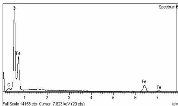
Fig. S3 Energy-dispersive X-ray spectroscopy (EDX) of  $\text{Fe}_3\text{O}_4$  nanowires.
