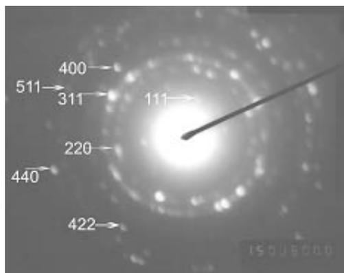
Fig. S4 Electron diffraction pattern of a  $\text{Fe}_3\text{O}_4$  nanowire
