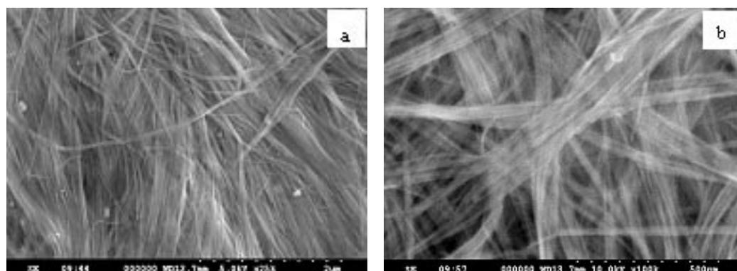
Fig. S2 SEM images of the magnetic nanowires prepared at P123/EG (0.50 wt%) in different magnifications.
