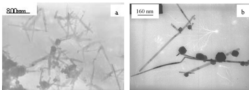
Fig. S1 TEM images of the magnetic nanowires prepared in different ratio of P123 and EG: (a) 0; (b) 20; wt %.
