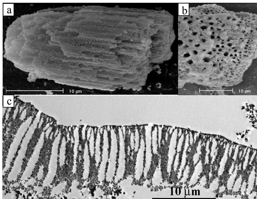
**Fig. 1** (a) SEM image of the as-synthesized ZrP-h sample; (b) SEM image of the calcined ZrP-hc650 sample; (c) cross-sectional TEM image of the ZrP-h sample. The hollow macrochannels are practically parallel to each other, and extend throughout almost the whole particles.
