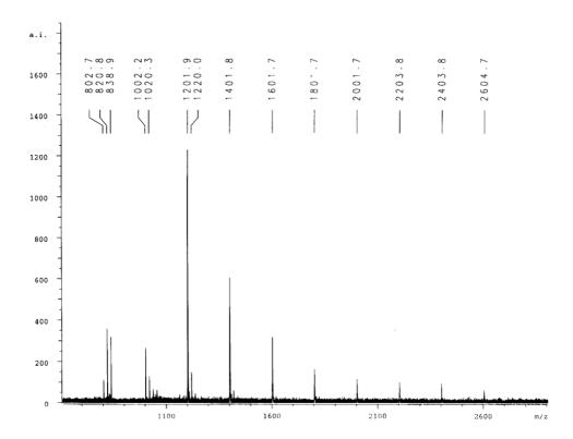
**Fig.** MALDI-TOF mass spectrum of polypyrene nanowires.
