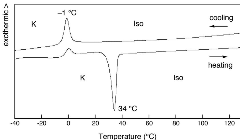
**Fig. S1** DSC trace on second heating/cooling cycle of **1b** (scan rate 10  $^{\circ}\text{C}$   $\text{min}^{-1}$ ). K, crystalline state; Iso, isotropic liquid.
