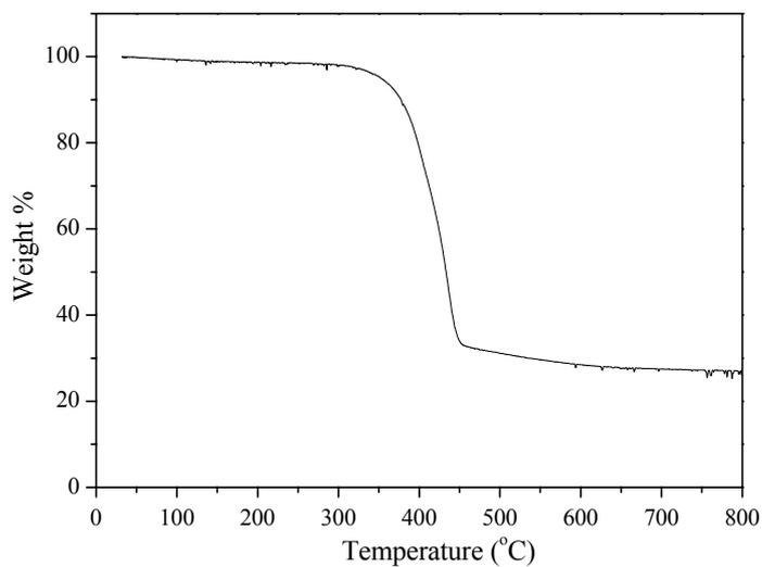
Fig. S2 The TGA of the as-synthesized HRP-IL@GEL.
