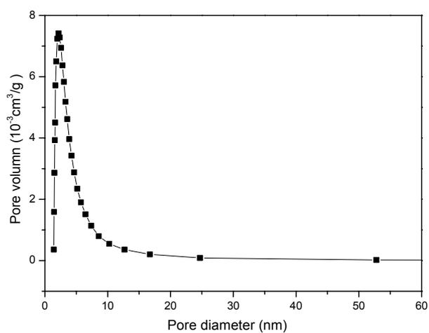
Fig. S3 The BJH desorption pore size distribution of the HRP-IL@GEL matrix after calcination.
