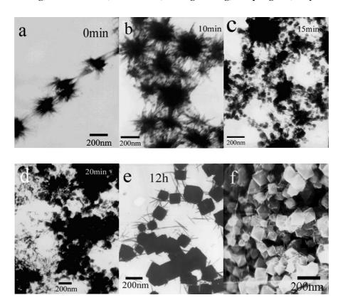
TEM and SEM images of five samples, showing different stages of growth for  $CeO_2$  nanocubes. (a)0 min; (b) 10min; (c) 15 min(d) 20min and (e, f) 12h.
