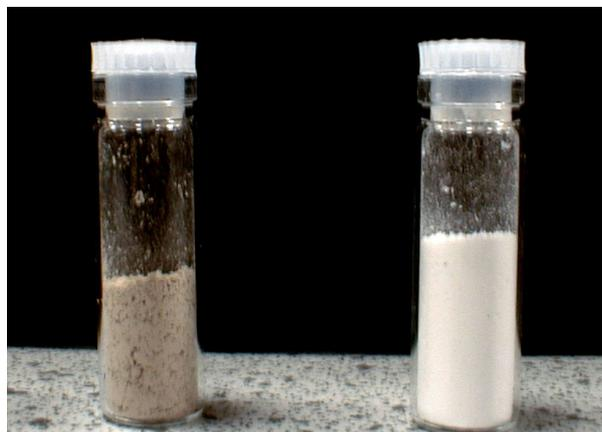
**Figure 1.** Polystyrene-C<sub>60</sub> composite microparticles: brown powder; and neat polystyrene microparticles: white powder.
